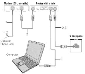
(Sample Illustration) 40/50L3400U Series - Connecting with Internet connection - wired
