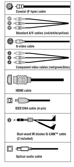
Note: Although your TV includes both HDMI and IEEE1394 connections, it may not operate with another device you have that includes such a connection. For example, the IEEE1394 ports are not intended to operate with current model Mini DV camcorders, and the HDMI input is not intended for connection to a computer. Copyright protection requirements may also prohibit or limit connectivity. See page 20 for details about the HDMI input. See pages 23–25 for details about the IEEE1394 ports.
