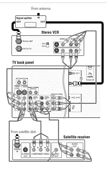
**Note:** The VIDEO/AUDIO OUT terminals output signals from the ANT 1, ANT 2, VIDEO 1, VIDEO 2, and VIDEO 3 terminals when the appropriate input mode is selected.
