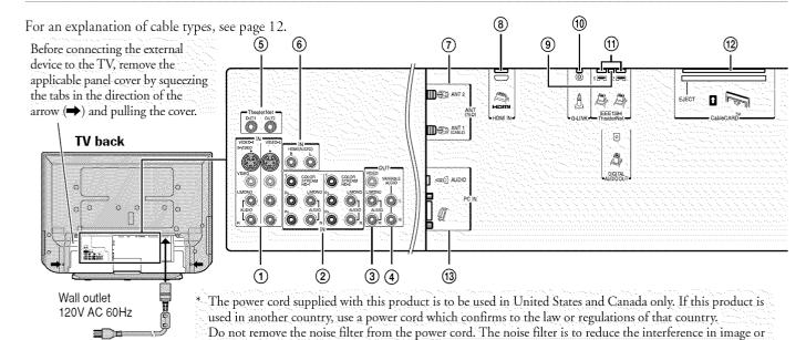
① **VIDEO 1 IN** and **VIDEO 2 IN** — Two sets of standard (composite) video and standard audio inputs plus optional S-video inputs for connecting devices with composite video or S-video output.
