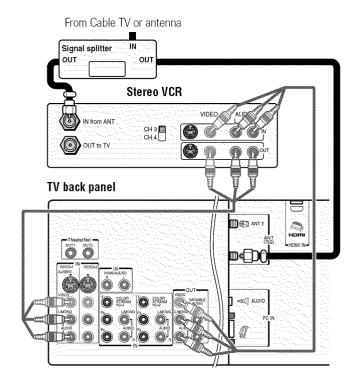
**Note:** The VIDEO/AUDIO OUT terminals output signals from the ANT 1, ANT 2, VIDEO 1, VIDEO 2, and VIDEO 3 terminals when the appropriate input mode is selected.
