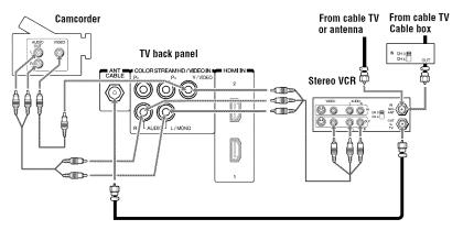
(Sample Illustration) 50L1450U—Connecting to a VCR, antenna, cable TV, or camcorder
