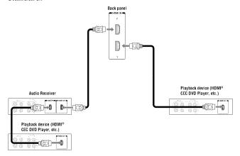
(Sample Illustration) 50L1450U— $HDMI^{\circ}$  CEC compatible audio receiver and playback device connections
