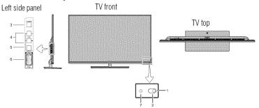
(Sample Illustration) 50L1450U - Front and side panel controls and connections
