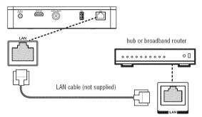
(Sample Illustration) Connecting to a wired router
