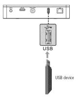
(Sample Illustration) Connecting a USB device
