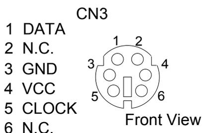
Figure 3-2 CN3: 6-Pin Mini Din Keyboard Connector
