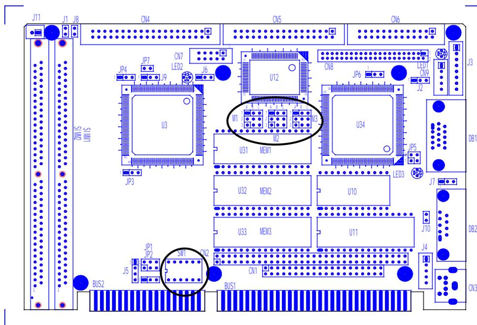
Figure 6-1 Switch & SSD Type Jumper Location
