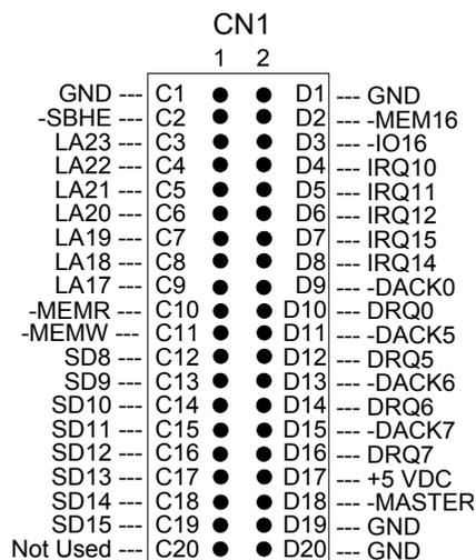
Figure 3-5 CN1: 40-Pin PC/104 Connector Bus C & D
