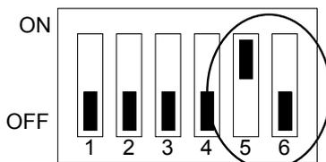
**Figure 6-6 5V Large FLASH (29FXXX) Switch Setting**
