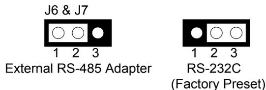
Figure 3-13 J6 & J7: External RS-485 Adapter Select
