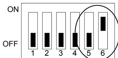
Figure 6-8 5V FLASH (29CXXX & 28EEXXX) Switch Setting
