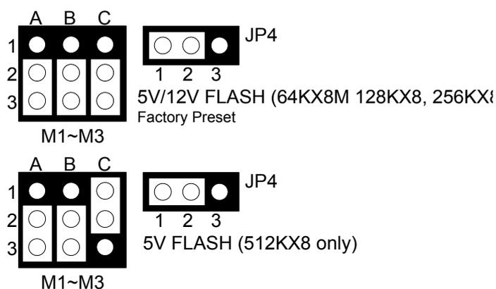
Figure 6-9 5V FLASH (29CXXX & 28EEXXX) Jumper Setting
