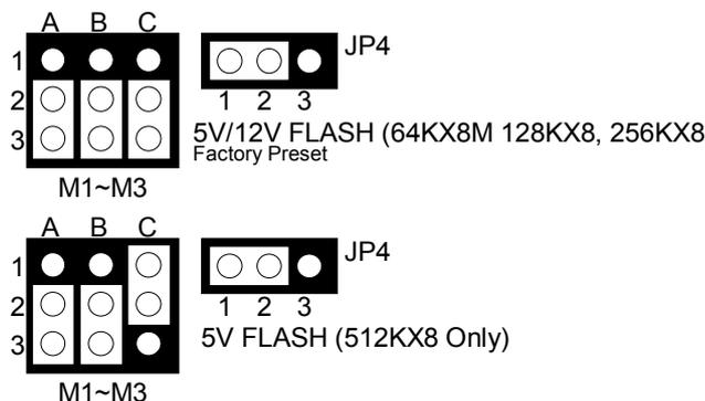
**Figure 6-7 Large Page 5V FLASH Jumper Setting**
