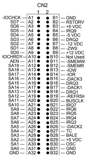
Figure 3-7 CN2: 64-Pin PC/104 Connector Bus A & B
