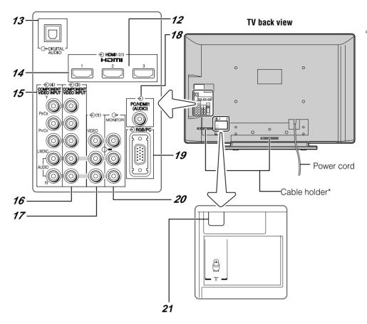
You can use the cable holder to hold aerial cable, video and audio cables etc.
