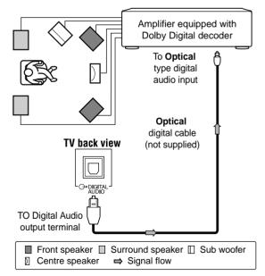
You can enjoy dynamic realistic sound by connecting the TV to an amplifier equipped with a Dolby Digital decoder or Dolby Digital processor. When using this setup, select **Auto** in the Digital Output menu.
