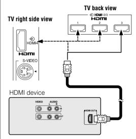
For proper operation, it is recommended that you use a short HDMI cable.
