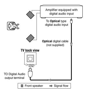
You can enjoy dynamic sound of 2-channel digital stereo by connecting the TV to an amplifier equipped with a digital audio (optical) input and speaker system (right and left front speakers). When using this setup, select **PCM** in the Digital Output menu.
