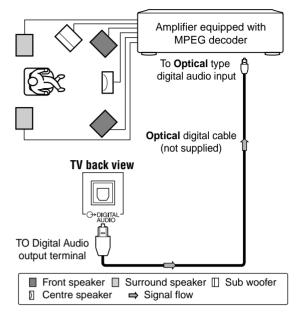
You can enjoy motion picture with dynamic realistic sound by connecting the TV to an amplifier equipped with an MPEG audio decoder or MPEG audio processor. When using this setup, select **Auto** in the Digital Output menu.
