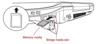
Figure 8-4 Inserting a memory media
