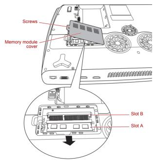
Figure 8-6 Removing the memory module cover
