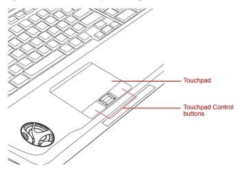
Figure 4-1 Touch Pad and Touch Pad control buttons
