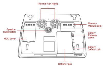
Figure 2-5 The underside of the computer
