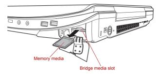
Figure 8-5 Removing memory media
