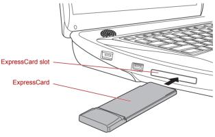
Figure 8-1 Inserting the ExpressCard
