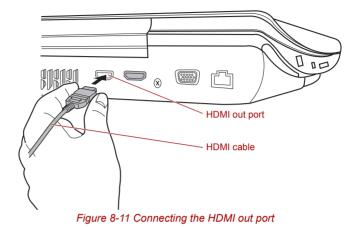
2. Plug the other end of the HDMI cable into the HDMI out port on your computer.
