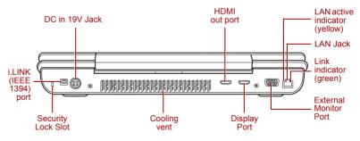
Figure 2-4 The back of the computer
