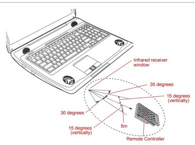
Figure 4-10 Operational range of the remote control
