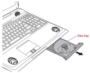
Figure 4-5 Pulling the disc tray open
