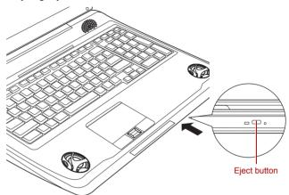
Figure 4-4 Pressing the eject button
