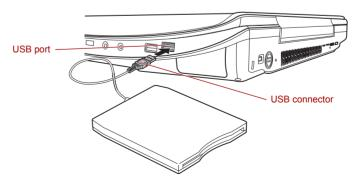
Figure 8-8 Connecting the USB floppy diskette drive
