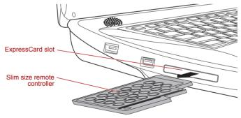
Figure 4-16 Removing a Slim size remote controller
