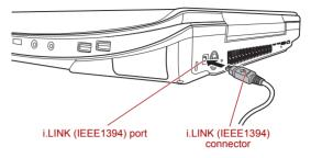
Figure 8-12 Connecting the i.LINK (IEEE1394) port
