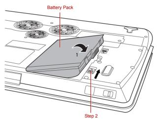
Figure 6-3 Securing the battery pack
