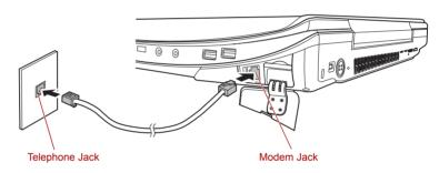
Figure 4-17 Connecting the internal modem
