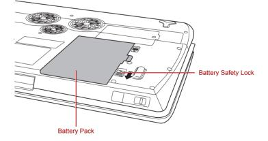
Figure 6-1 Releasing the battery pack (1)
