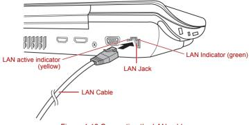
Figure 4-18 Connecting the LAN cable
