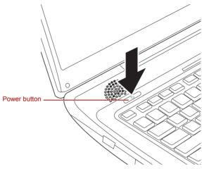
Figure 3-4 Turning on the power
