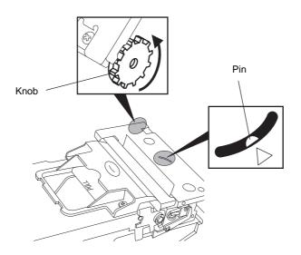
3) Remove the jammed paper. DO NOT USE any sharp implement or tool as these will damage the printer.
