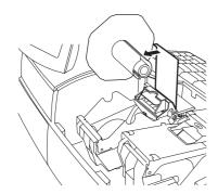
7. Insert the paper end into the slit of the Take-up Reel and wind it around the reel twice or three times.
