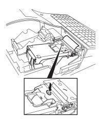
4. Pull the end of receipt roll forward until the area with the glue on the paper is past the Cutter Block.
