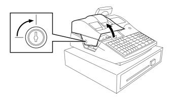
1. To remove the Printer Cover, insert the Printer Cover Key to the Printer Cover Lock, and then turn it 90° clockwise.
