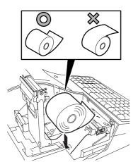
2. Pull up the Printer Release Lever to open the Receipt Cover Frame Ass'y.
