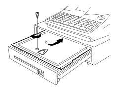
2) Press the cover lightly, insert the key into the key hole on the cover, and turn it 90° clockwise.
