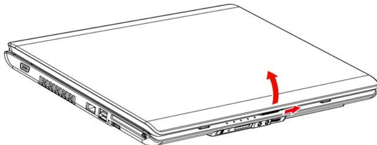
Figure 3-3 Opening the display panel
