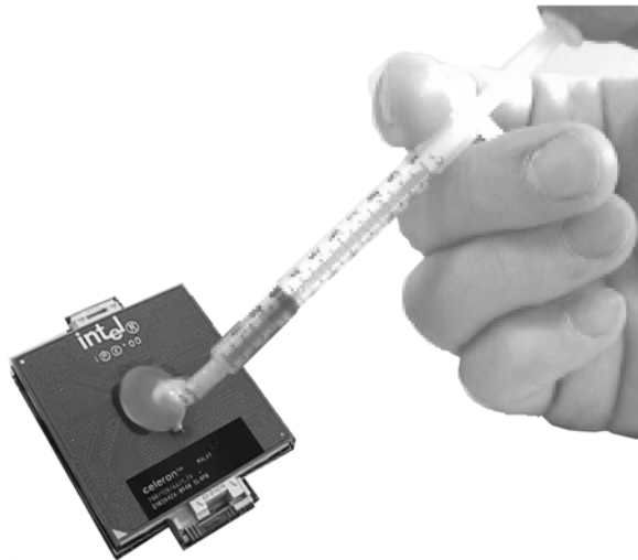
Figure 4-17 Applying new grease
