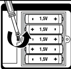
1. To remove battery cover, loosen screw to open.
