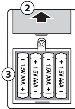
1. To remove battery lid, loosen screw to open.
