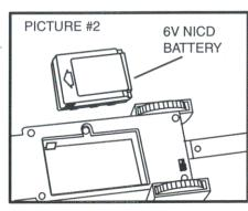
Reinstell the battery compartment door. Secure with the screw.
