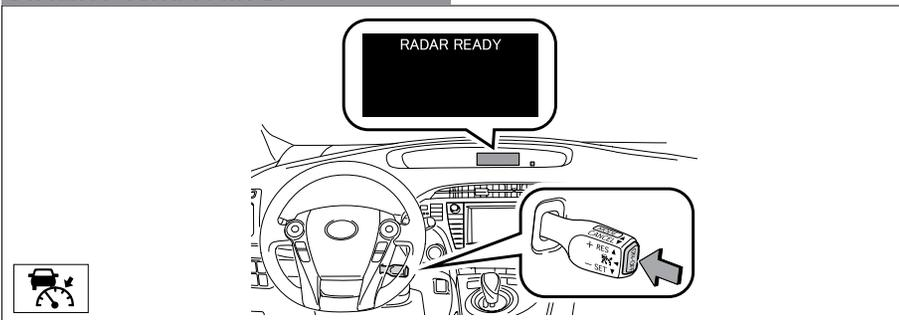
In distance control mode, vehicle will cruise at a set speed, decelerate to maintain selected distance from a slower vehicle traveling in front, and accelerate back up to the selected speed if the vehicle in front changes lanes or speeds up.
