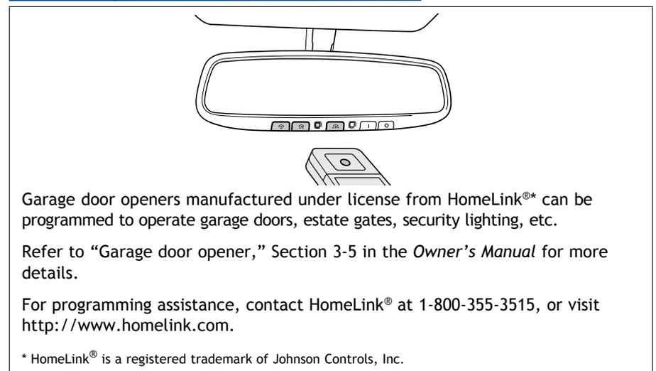
Garage door openers manufactured under license from HomeLink®\* can be programmed to operate garage doors, estate gates, security lighting, etc.
