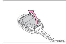
3 Open the case cover using a coin protected with tape, etc., and remove the depleted battery using a small flathead screwdriver.
