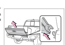
3 Slide the tailgate a little to the right to unhook the left side being mindful of tailgate right-hand side clearance to vehicle's rear bumper.
