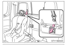
4 Latch the hook onto the anchor bracket and tighten the top tether strap.
