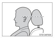
Adjusting the rear center seat head restraint (Double Cab models only) Always raise the head restraint one level from the stowed position when using.
