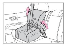
5 If the child restraint has a top tether strap, the top tether strap should be latched onto the top tether strap anchor. (→P. 63, 65)
