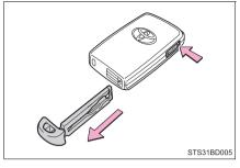
After using the mechanical key, store it in the electronic key. Carry the mechanical key together with the electronic key. If the electronic key battery is depleted or the entry function does not operate properly, you will need the mechanical key.  $(\rightarrow P. 555)$
