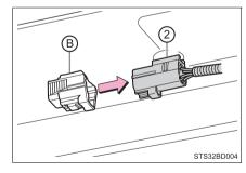
Pull out the plastic wire protector located in the vehicle bed by pressing the tabs and pulling the protector.
