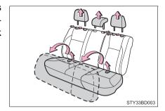
Attach the head restraints to the holders located on the back sides of the bottom cushions.
