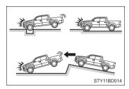
The SRS curtain shield airbags may also deploy under the situation shown in the illustration.
