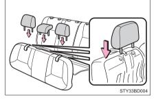
Center head restraint: The front of the head restraint facing forward.
