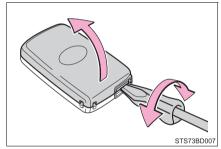
Remove the depleted battery.
