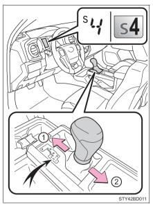
The initial shift range in S mode is set automatically to 5 or 4 according to vehicle speed. However, the initial shift range may be set to 3 if the AI-SHIFT has operated while the shift lever was in the D position.  $(\rightarrow P. 198)$
