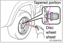
▶ Replacing an aluminum wheel with a spare aluminum wheel
