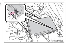
Under the instrument panel Remove the cover.
