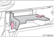
4 Remove the cover by sliding up and then pull the cover toward you.
