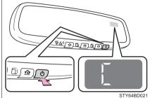
Drive the vehicle at 5 mph (8 km/h) or less in a circle until a direction is displayed.
