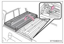
4 Secure by using the storage straps.
