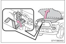
3 Hold the hood open by inserting the supporting rod into the slot.
