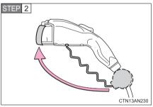
Attach the charging connector cap.
