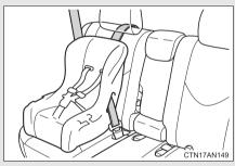
Seat belts equipped with a child restraint locking mechanism (ALR/ELR belts except driver's seat belt) (→P. 134)
