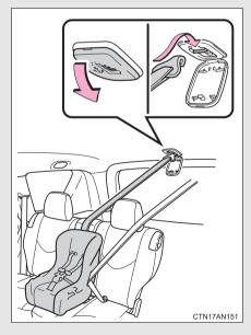
Rear center seat: Anchor bracket (for top tether strap)
