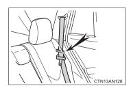
Pass the outer rear seat belts through the seat belt hangers and secure the seat belt plates to prevent the shoulder belts from being damaged.
