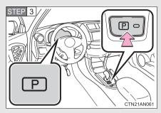
Push the P position switch to shift into P.  $(\rightarrow P. 209)$
