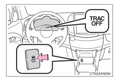
To turn the TRAC system off, quickly press and release  $\frac{1}{2}$ .
