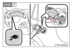
Confirm the charging cable connector's direction and insert it into the charging port.
