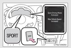
By increasing the motor's output when compared to normal mode, the vehicle's acceleration power and maximum speed is increased. This mode provides a more dynamic driving experience.
