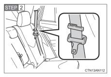
Make sure the outside seat belt passes through the hanger when folding the rear seat.
