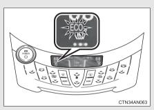
When the air conditioning is set to ECO LO or ECO HI mode, the seat heater is automatically operated and its temperature automatically adjusted according to the outside temperature and air conditioning settings.
