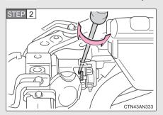
Using a Phillips-head screwdriver, turn bolt A in either direction.
