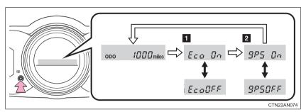
While the odometer is being displayed, customization can be performed by pressing and holding the display change button.
