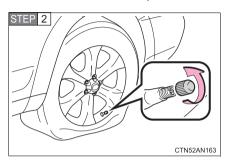
Remove the valve cap from the valve of the punctured tire.
