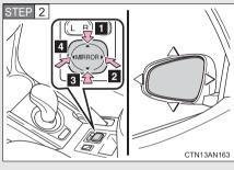
To adjust the mirror, press the switch.
