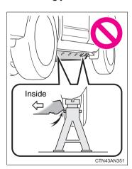
When lowering the vehicle onto jack stands, do not let the jack stands contact the traction battery or undercover. Doing so may damage the vehicle underbody. Working on the vehicle while a jack stand is contacting the traction battery is particularly dangerous because it may not only damage the traction battery, but the vehi-
