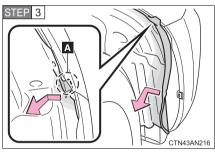
Move section "A" of the fender liner to the inner side of the vehicle, partly removing it and thereby allowing access to the front turn signal.
