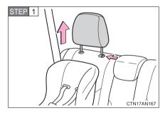
Remove the head restraint.
