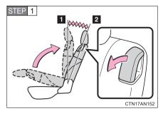
Fold the seatback while pulling the lever. Return the seatback and secure it at the 1st lock position (most upright position). Adjust the seatback to the 7th lock position. (→P. 121)
