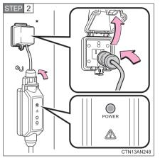
Insert the charging cable's plug into the electrical receptacle of the external power source.
