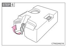
Lift the rubber stopper on the compressor.
