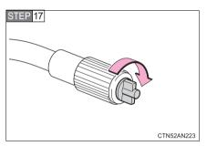
Attach the air release cap to the end of the hose.
