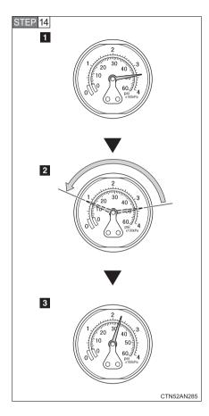
Inflate the tire until the specified air pressure is reached.
