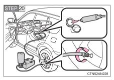
After driving for about 3 miles (5 km), stop your vehicle in a safe place on a hard, flat surface and remove the air release cap from the hose before reconnecting the repair kit.
