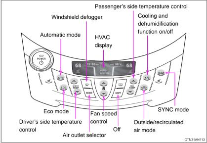
The operating section of the air conditioning panel uses capacitive touch sensors. ( $\rightarrow$ P. 290)
