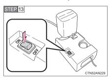
To inject the sealant and inflate the tire, turn the compressor switch on.
