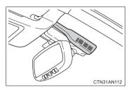
In order to detect fog on the windshield, a sensor which monitors the temperature of the windshield, the surrounding humidity, etc. is installed.  $(\rightarrow P.~286)$
