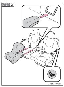
Latch the buckles onto the LATCH anchors.
