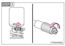
Extend the hose. Remove the air release cap from the hose.
