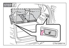
Open the back door and pull the lock release lever to fold down the rear seat.
