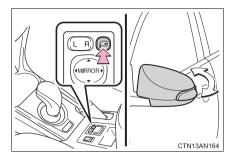
Press the switch to fold the mirrors.
