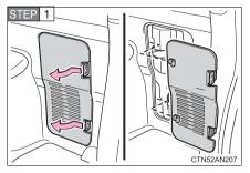
Disengage the claws and remove the cover.
