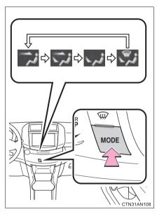
Manual mode: The air outlets switch each time MODE is pressed.
