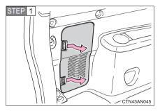
Open the back door ( $\rightarrow$ P. 113) and remove the cover.
