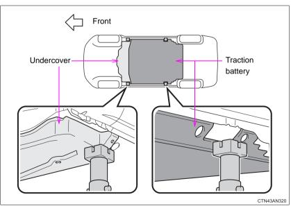
Before lowering the vehicle onto jack stands, check that the jack stands will not contact the traction battery or undercover.
