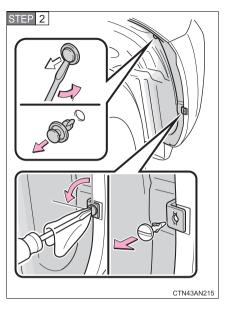
Remove the clips using a flathead screwdriver.
