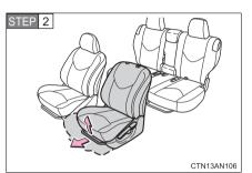
Slide the front seat further forward than the forward-most lockable position.
