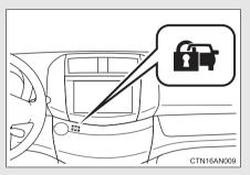
The indicator light flashes after the "POWER" switch has been turned off to indicate that the system is operating.
