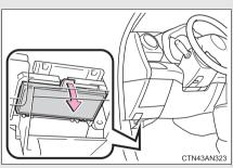
Fuse block (under side view): Remove the lid.
