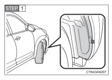
Turn the steering wheel in the opposite direction of the front turn signal that you wish to replace.
