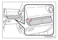
To open and close the auxiliary box, press the button.
