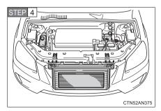
After "High Battery Temp" disappears, check the motor/traction battery coolant level and inspect the cooling system for leaks.
