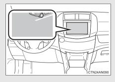
The rear view image is displayed when the shift position is in R.
