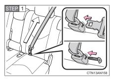
To release tab "A", insert tab "B" or the mechanical key ( $\rightarrow$ P. 94) into the hole on the buckle.
