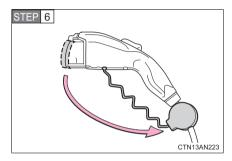
Remove the charging connector cap.
