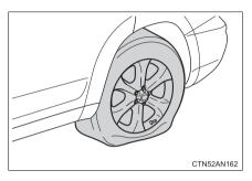
A tire should only be repaired with the emergency tire puncture repair kit if the damage is caused by a nail or screw passing through the tire tread.
