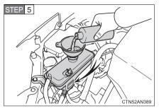
If necessary, add motor coolant up to the "FULL" line.
