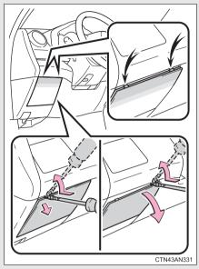
Front side of the fuse block: Remove the cover.
