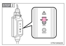
Press the test button on the CCID (Charging Circuit Interrupting Device).
