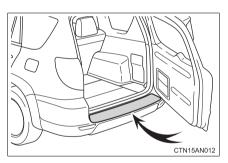
The rear step bumper is intended for rear end protection and easier step-up loading.
