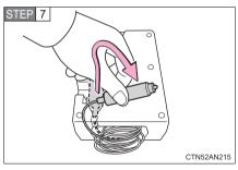
Remove the power plug from the compressor.
