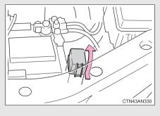
Type C: Push the tab in and lift the lid off.
