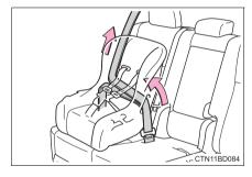
6 If the child restraint has a top tether strap, the top tether strap should be latched onto the top tether strap anchor. (→P. 75)
