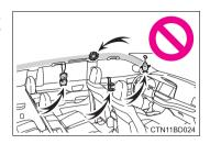
Vehicles without a smart key system: Do not attach any heavy, sharp or hard objects such as keys and accessories to the key. The objects may restrict the SRS driver's knee airbag inflation or be thrust into the driver's seat area by the force of the deploying airbag, thus causing a danger.
