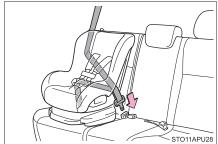
4 Fully extend the shoulder belt and allow it to retract to put it in lock mode. In lock mode, the belt cannot be extended.
