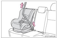
6 If the child restraint has a top tether strap, the top tether strap should be latched onto the top tether strap anchor. (→P. 63)
