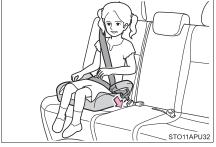
Check that the shoulder belt is correctly positioned over the child's shoulder and that the lap belt is as low as possible.  $(\rightarrow P. 26)$
