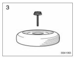
3. Loosen the bolt and remove it.
