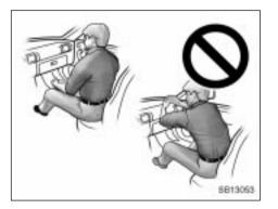
• Do not sit on the edge of the seat or lean over the dashboard when the vehicle is in use. When the airbags inflate with considerable speed and force; Otherwise, you may be killed or seriously injured. Sit up straight and well back in the seat, and always use your seat belt properly.
