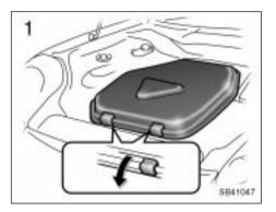
To remove the compact spare tire: 1. Open the front box cover in the trunk.
