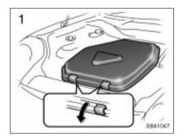
To remove the compact spare tire: 1. Open the front box cover in the trunk.
