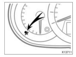
This indicator comes on when the ignition key is turned to the "ON" position. It goes off after about 6 seconds. This means the seat belt pretensioners are operating properly.
