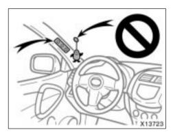
• Do not attach a microphone or any other device or object near the area where the curtain shield airbag activates such as on the windshield glass, side door glass, front, center and roof side garnish. When the curtain shield airbag inflates, the microphone or other device or object will be thrown away with great force or the curtain shield airbag may not activate correctly, resulting in death or serious injury.
