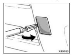
Remove the front towing eyelet cover on the front bumper, using a flathead screwdriver which is wrapped with a cloth.
