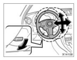
To adjust the steering wheel position, push down the lock release lever. Then tilt the steering wheel to the desired angle, push or pull it to the desired steering column length and return the lever to its original position.
