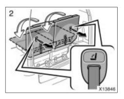
2. Pull the seatback lock release strap to fold down the seatback. Make sure it is locked securely.
