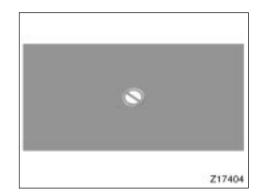
If " $\circ$ " appears on the screen when you select a switch, it indicates that the switch cannot work.
