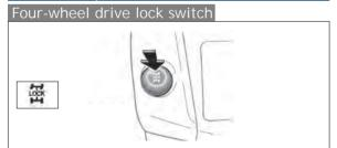
Push the switch to ensure that the engine torque is applied to the 4 wheels.
