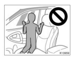
• Do not allow anyone to kneel on the passenger seat, facing the passenger's side door, since the side airbag and curtain shield airbag could inflate with considerable speed and force. Otherwise, he/she may be killed or seriously injured. Special care should be taken especially when you have a small child in the vehicle.
