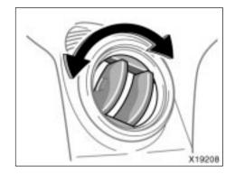
You can change air flow direction by turning the side vents.
