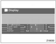
Operate the joystick up and down to select Brightness, Contrast, Tone, or Color
