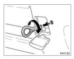
Use the front towing eyelet in the tool bag. Secure it to the hole on the bumper by turning clockwise. (For the tool bag location, see "—Required tools and spare tire" on page 326 in this Section.)
