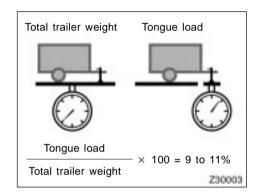
Never load the trailer with more weight in the back than in the front. About 60% of the trailer load should be in the front half of the trailer and the remaining 40% in the rear.
