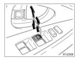
The windows can be operated with the switch on each door. The passengers' windows can also be controlled by the switches on the driver's door.
