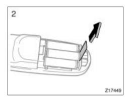
2. Remove the insulating sheet.
