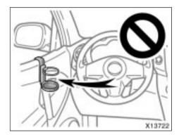
• Do not attach a cup holder or any other device or object on or around the door. When the side airbag inflates, the cup holder or any other device or object will be thrown with great force or the side airbag may not activate correctly, resulting in death or serious injury. Likewise, the driver and front passenger should not hold objects in their arms or on their knees.
