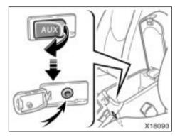
An AUX adapter is installed in the rear console box.
