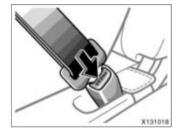
To remove the booster seat, press the buckle release button and allow the belt to retract.
