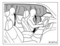
The SRS (Supplemental Restraint System) side airbags and curtain shield airbags are designed to provide further protection for the driver, front passenger and rear/second passengers in addition to the primary safety protection provided by the seat belts.
