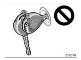
♦ When starting the engine, do not use the key with other transponder keys around (including keys of other vehicles) and do not press other key plates against the key grip. Otherwise the engine may not start, or may stop soon after it starts. If this happens, remove the key once and then insert it again after removing other transponder keys (including keys of other vehicles) from the ring or while gripping or covering them with your hand to start the engine.
