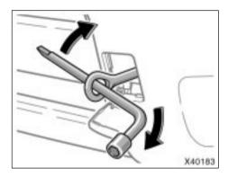
3. Tighten the front towing eyelet securely by a wheel nut wrench.
