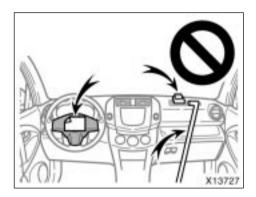
• Do not put anything or any part of your body on or in front of the dashboard or steering wheel pad that houses the front airbag system. They might restrict inflation or cause death or serious injury as they are projected rearward by the force of the deploying airbags. Likewise, the driver and front passenger should not hold objects in their arms or on their knees.
