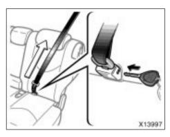
Rear/second center seat: If the seat in which a child restraint system is installed in the rear most position, release the center seat belt after removing the child restraint system. Otherwise, the rear center seat belt may not work properly.
