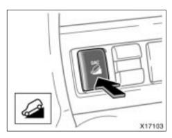
2. Push the "DAC" switch to turn the system on. The downhill assist control system indicator light will come on
