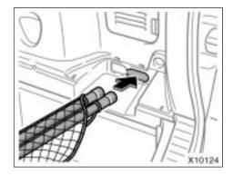
3. Insert the right end of the rear cargo net into the luggage storage box as shown.
