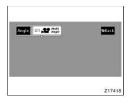
The angle can be selected for discs that are multi-angle compatible when the "AT" mark appears on the screen. Each time you push the "Angle" switch, the angle changes. The angle number which you can select will appear on the screen.
