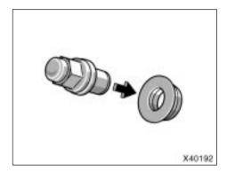
On vehicles with aluminum wheels and a steel wheel for the spare, remove the rubber rings from the wheel nuts of the spare tire carrier before stowing a flat tire. Be careful not to lose the rubber rings after removing them.
