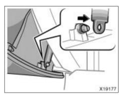
1. Open the glove box. Slide off the damper as shown.
