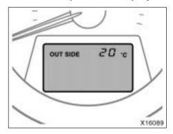
The displayed temperature ranges from -40°C (-40°F) up to 50°C (122°F).
