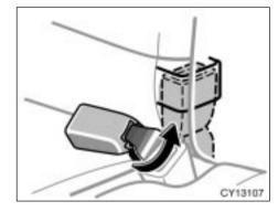
BEFORE FOLDING DOWN REAR SEAT Stow the rear center seat belt buckle as shown in the illustration.
