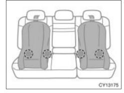
Lower anchorages for the child restraint systems complying with the FMVSS225 or CMVSS210.2 specifications are installed in the rear seats.
