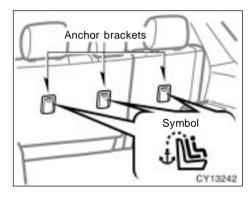
Use the anchor brackets behind the second seatbacks to attach the top strap.
