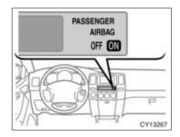
The front passenger occupant classification indicator light indicates the actuation of the front passenger airbag, side airbag on the front passenger seat and front passenger's seat belt pretensioner.
