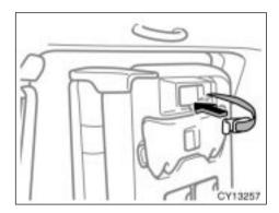
When returning the third seat to its original position, stow the holding strap in the holder in the direction shown above. Then do the above procedures in the reverse order.
