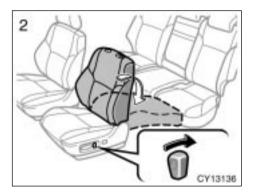
2. Move the seatback angle adjusting switch backward to flatten the seatback.
