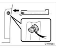
If the trash holder is pulled strongly or stepped on, it will detach from the rear console box to protect it from damaging.
