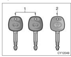
To protect items locked in the glove box when using valet parking, leave the sub key with the attendant.
