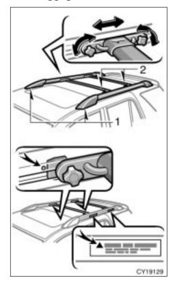
The roof luggage carrier consists of roof rails (1) attached to the roof and sliding cross rails (2).
