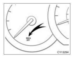
The seat belt pretensioners will not operate in a vehicle rollover if the "RSCA OFF" indicator light is on. For details, see "Roll sensing of curtain shield airbags off switch" on page 95 in this Section.
