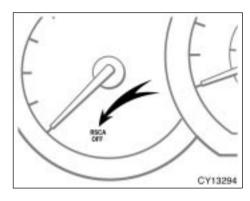
• Make sure the "RSCA OFF" indicator light is off. The curtain shield airbags will not inflate in a vehicle rollover if this indicator light is on and you may be killed or seriously injured. For details, see "Roll sensing of curtain shield airbags off switch" on page 95 in this Section.
