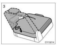
3. Raise the seatback while pushing down the seatback angle adjusting lever.
