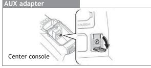
By inserting a mini plug into the AUX audio jack, you can listen to music from a portable audio device through the vehicle's speaker system.
