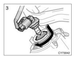
3. Install a new bulb and connector into the mounting hole and turn them clockwise to the front of the vehicle. 06 06.07
