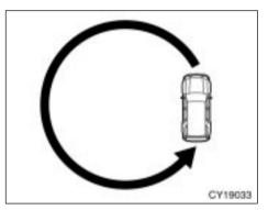
Drive the vehicle in a circle at 8 km/h (5 mph) or less. If there is not enough space to drive in a circle, drive around the block.
