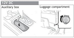
**NOTE:** Designed for car accessories. Key must be in the "ACC" or "ON" position to be used.
