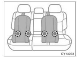
Lower anchorages for the child restraint systems complying with the FMVSS225 or CMVSS210.2 specifications are installed in the second seats.
