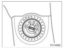
For easy access to the ignition switch, the ignition switch light comes on when any of the side doors and back door is opened or when the ignition switch is turned to the "LOCK" position.
