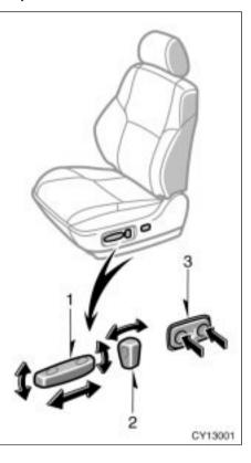
1. DRIVER'S SEAT: SEAT POSITION, SEAT CUSHION ANGLE AND SEAT HEIGHT ADJUSTING SWITCH PASSENGER'S SEAT: SEAT POSITION ADJUSTING SWITCH
