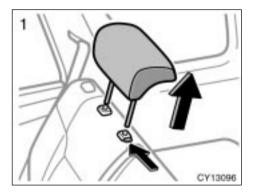
TO USE THE ANCHOR BRACKET: 1. Remove the head restraint.
