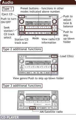
To scan tracks on a disc Push "SCAN." Push again to hold selection.
