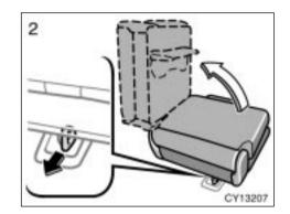
2. Unlock the seat leg by pulling the handle behind the seat, and swing the whole seat up and sideward.
