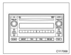
Type 2: AM-FM radio/compact disc player with changer (with XM<sup>®</sup> satellite radio<sup>\*</sup> controller)
