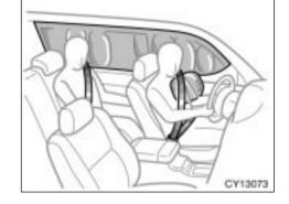
The SRS (Supplemental Restraint System) side airbags and curtain shield airbags are designed to provide further protection for the driver, front passenger and rear seat passengers<sup>\*1</sup>/second seat passengers<sup>\*2</sup> in addition to the primary safety protection provided by the seat belts.
