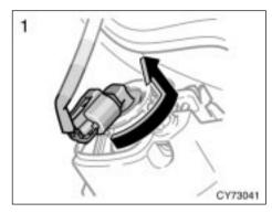
1. Turn the bulb base counterclockwise to the front of the vehicle as shown.
