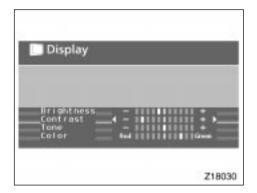
Operate the joystick up and down to select Brightness, Contrast, Tone, or Color and left and right to make adjustments.
