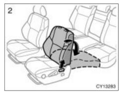
2. Pull the seatback angle adjusting lever to unlock and push down the seatback.
