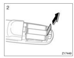
2. Remove the insulating sheet.
