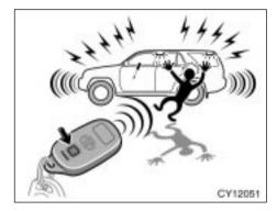
Pushing the "PANIC" switch blows the horn intermittently and flashes the headlights, tail lights and turn signal lights, and turns on the interior and luggage compartment lights.
