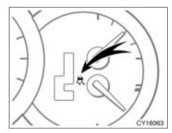
When the hill-start assist control system is operating, the slip indicator light flashes and an alarm sounds intermittently. At the same time, the stop lights and high mounted stoplight are lit.
