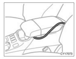
After plugging the cord into the adapter, let it go through the gap between the console box and the tray. Use a cord which is thin enough to go through the gap. Close the console box lid.
