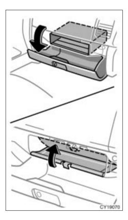
On some models, an auxiliary box is located inside the glove box.
