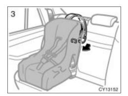
3. Fix the child restraint system with the seat belt.
