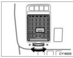
If air flow control is not satisfactory, check the instrument panel and rear vents. The instrument panel and rear vents may be opened or closed as shown.
