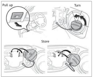
**NOTE:** Tighten until one click is heard. If the cap is not tightened enough, Check Engine " $\bigotimes_{max}$ " indicator may illuminate.
