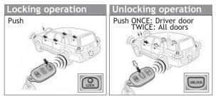
**NOTE:** After unlocking, if a door is not opened within 30 seconds, all doors will relock for safety.
