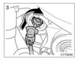
3. Install a new bulb and connector into the mounting hole and turn them clockwise to the front of the vehicle.
