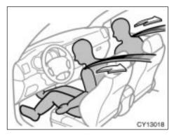
The driver and front passenger seat belt pretensioners are designed to be activated in response to a severe frontal impact. On vehicles equipped with curtain shield airbags, the pretensioners are also activated during vehicle rollover.
