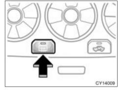
To defog or defrost the back window, push the switch with the back window closed.
