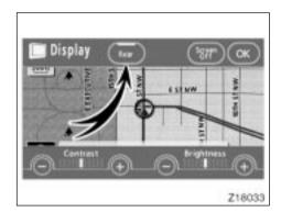
Vehicles with navigation system—The rear seat entertainment system can be switched ON and OFF by pushing the "Rear" switch on the front audio system.
