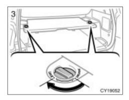
3. Turn the left and right knobs from the "UNLOCK" position to the "LOCK" position.
