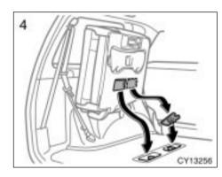
4. Remove the seat anchor covers from the back of the seat cushion, and install them over the seat anchors.
