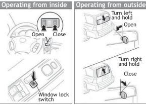
**NOTE:** If the battery is disconnected, the rear hatch window will need to be reinitialized. Refer to the *Owner's Manual* for more details.
