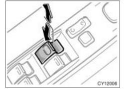
Automatic operation: Push the switch completely down or pull it completely up, and then release it. The window will fully open or close. To stop the window partway, lightly move the switch in the opposite direction and then release it.
