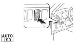
Push the "AUTO LSD" switch when the vehicle is stopped. To deactivate, push the switch again.
