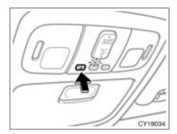
5. Test the operation of the HomeLink<sup>®</sup> by pressing the newly programmed button. If programming a garage door opener, check to see if the garage door opens and closes.
