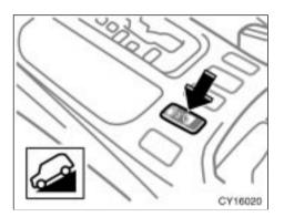
Multi-mode four-wheel drive models—If the downhill assist control system indicator light flashes, the selector lever may be in "N" or the multi-mode control switch knob may be in the "H2" or "H4" position.
