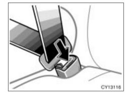
4. To remove the infant seat, press the buckle release button and allow the belt to retract completely. The belt will move freely again and be ready to work for an adult or older child passenger.
