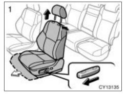
1. Remove the head restraint. Move the seat position adjusting switch forward to slide the seat further forward than the front-most position.
