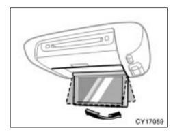
Pull the display down to an easily viewable angle (between  $90^{\circ}$  and  $125^{\circ}$ )
