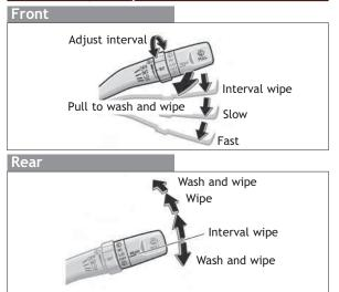
NOTE: Rear wiper and washer operate only when rear window is fully closed. If battery is disconnected, rear washer will not function until rear window is reinitialized by being fully opened and then closed.
