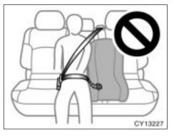
• When using the left side lower anchorages for the child restraint system, do not sit in the center seat. The performance of the center seat belt cannot be brought out sufficiently because the belt may be high-positioned or the seat belt may be loose-fitting, posing the risk of serious injury in the case of collision.
