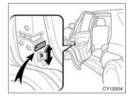
REAR DOOR CHILD-PROTECTORS Move the lock lever to the "LOCK" position as shown on the label.
