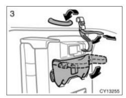
3. Stow the seat leg in the back of the seat cushion. Take the holding strap out of its holder, and attach the strap to the assist grip. Tighten the strap by pulling the end and fix it with Velcro.
