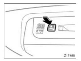
EJECTING THE DISC Push the "**≜**" button.
