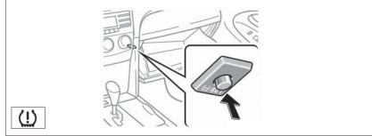
If tire pressure becomes low on any of the tires (including spare/excluding compact spare), indicator comes on. Pushing reset button should not turn off the light. Correctly adjusting tire inflation will turn off the light after a few minutes. Push and hold reset button, until the indicator light blinks 3 times, after replacing tire or wheels.
