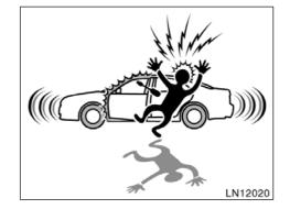
To deter vehicle theft, the system is designed to sound an alarm if any of the doors, trunk or hood is forcibly unlocked or the battery terminal is disconnected and then reconnected when the vehicle is locked.
