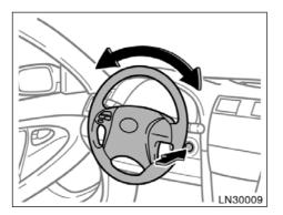
If the green indicator light on the "ENGINE START STOP" switch flashes, and the "S/T IS NOT UNLOCKED" message appears on the multi-information display and the master warning light comes on, the steering wheel is locked.
