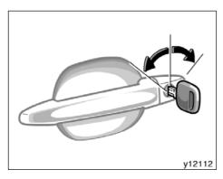
When either front door is unlocked with a key, the front personal lights and engine switch light will come on and remain on for about 15 seconds before fading out. (For details, see "Front personal lights" on page 179 and "Engine (ignition) switch light" on page 181 in Section 1–5.)
