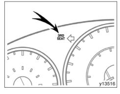
This "3RD SEAT" warning light warns the third seat operation is not yet complete when the engine switch is turned to the "ON" position.
