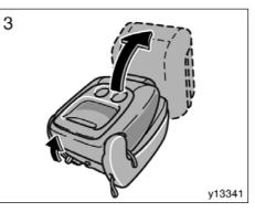
3. Pull the seat lock release lever (red) and swing up the seat.
