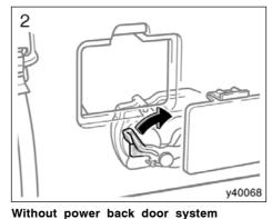
If the back door opener does not operate, you can open the back door from the inside.
