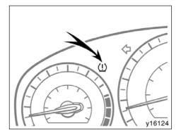
The tire pressure warning light comes on when the engine switch is in "ON" position and goes off after a few seconds. This means the tire pressure warning system is operating properly. If the tire inflation pressure becomes low, the light comes on again. In this case, adjusting the tire inflation pressure will turn off the light after several minutes. If the light comes on after blinking for 1 minute, the tire pressure warning system is not working properly.
