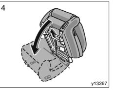
4. Pull and hold the front leg release strap and fold down the seat. Then the front leg locks will disengage and you can remove the seat.
