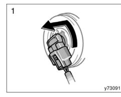
1. Open the hood. Press the bulb base slightly and turn the bulb base counterclockwise to the front of the vehicle as shown.
