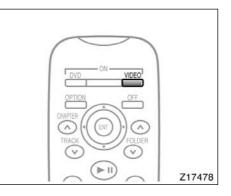
The audio machine connected to the input terminal adapter can be played in the video mode.
