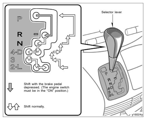
Your automatic transmission has a shift lock system to minimize the possibility of incorrect operation. This means you can only shift out of "P" position when the brake pedal is depressed (with the engine switch in the "ON" position).
