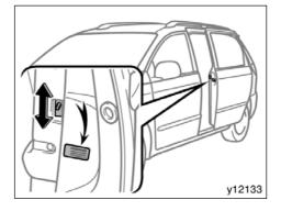
Open the sliding door fully and move the lock lever to the "LOCK" position as shown on the label. Then close the sliding door.
