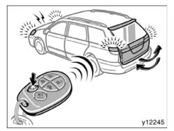
Push and hold the back door open switch on the wireless remote control transmitter for about one second. The power back door opens and closes completely.
