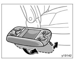
To fold down the table, pull up the lock release lever and push against the driver's seat side.
