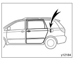
When the fuel filler door is opened, the left side sliding door will not open. Close the fuel filler door securely and then operate the sliding door.
