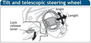
Hold wheel, push lever down, set angle and length, and return lever.
