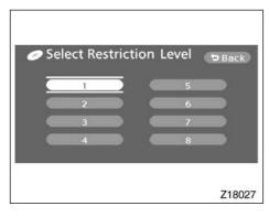
Select a parental level (1—8). The smaller the level number, the stricter the age limit. Select the "Back" switch to return to the "Setup Menu" screen.
