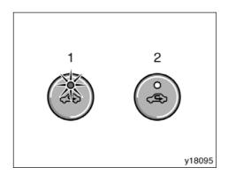
If the ambient temperature drops, the air intake mode will automatically change from RECIRCULATE to FRESH after a few minutes. This automatic change control mode can be cancelled by pushing and holding the button for longer than 2 seconds. The automatic change control mode will be reactivated if the engine switch is turned to the "LOCK" or "ACC" position.
