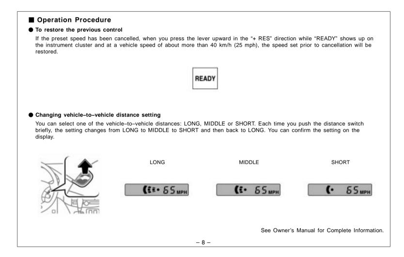
In addition to the vehicle-to-vehicle distance control mode described in this quick reference guide, dynamic laser cruise control has conventional (fixed speed) cruise control mode for cruising at fixed speeds. For the conventional cruise control mode, see Section 1–7 in the "Owner's Manual".
