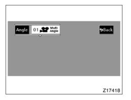
The angle can be selected for discs that are multi-angle compatible when the "P" mark appears on the screen. Each time you push the "ENT" button after selecting the "Angle" switch, the angle changes. The angle number which you can select will appear on the screen.
