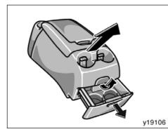
To remove the console box: Open the auxiliary box of the rear side and pull up the lock release lever to disengage the rear lock. Then lift the console box and release the front hook.
