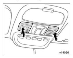
To turn on the front personal lights, operate the personal light main switch. The lights can be turned on or off by pushing each lens when the personal light main switch is in the "DOOR" or "OFF" position.
