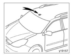
The compass sensor is on the roof of the vehicle.
