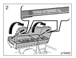
2. Pull the seatback angle adjusting strap ("TO FOLD/LIFT SEATBACK" printed on its surface) and raise the seatback.
