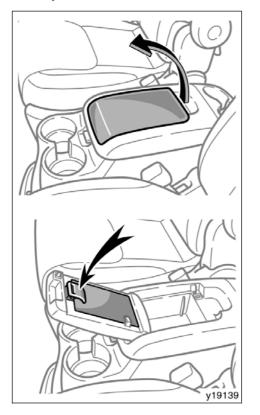
The note pad holder is designed to hold small paper such as note pads. To use the holder, raise the console box upper lid.
