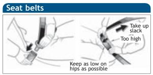
If belt is fully extended, then retracted even slightly, it cannot be re-extended beyond that point, unless fully retracted again. This feature is used to help hold child restraint systems securely.
