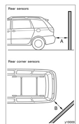
This system is designed to inform you of the approximate distance between your vehicle and an obstacle by indicator and buzzer.
