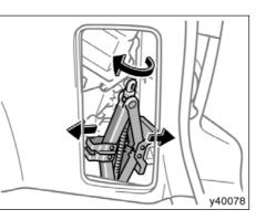
To store the jack, turn the jack joint until the jack base fits securely with the vehicle body.
