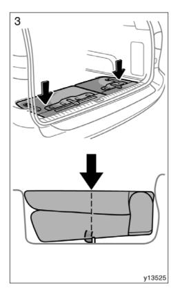
3. Push the seat against the floor and make sure it is locked securely.
