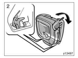
2. Make sure the front leg is locked securely, fold down the seat and engage the rear leg lock.
