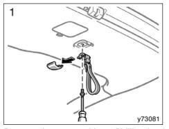
Remove the strap with a Phillips-head screwdriver.
