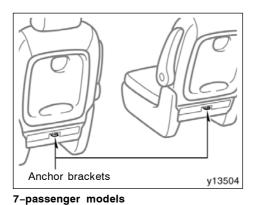
Use the anchor brackets on the back of the second seats to attach the top strap. Anchor brackets are installed for each second seating position.
