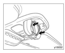
The mirror angle can be adjusted by pushing its edge.
