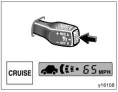
Vehicle-to-vehicle distance control mode
