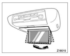
Pull the display down to an easily viewable angle (between  $90^{\circ}$  and  $125^{\circ}$ )
