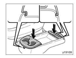
To install the cup holder and small tray: Cup holder—Hook the front of the cup holder to the console box under-tray, then push down the back of the cup holder to secure it.
