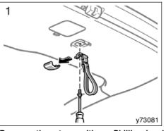
Remove the strap with a Phillips-head screwdriver.
