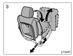
3. Fold down the seatback while pulling the seatback angle adjusting lever or strap and swing up the seat.
