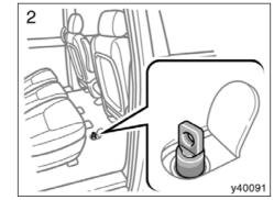
2. Attach the adapter socket over the spare tire clamp bolt.
