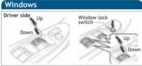
Automatic operation\* (driver side only) Push the switch completely down or pull it completely up and release to fully open or close. To stop window midway, lightly push the switch in the opposite direction.
