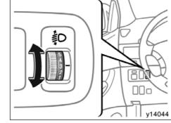
To adjust the headlight beam level, turn the dial.
