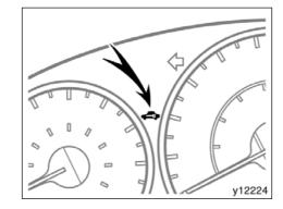
The system is automatically set when the key is removed from the engine switch.
