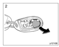
2. Remove the discharged transmitter battery.
