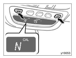
2. Push and hold both the "MODE" and "E/M" buttons simultaneously for 10 seconds until the "CAL" indication appears on the compass display. (At this time, the compass display is locked in "N".)
