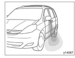
The light will come on when the side doors and back door are unlocked simultaneously using either the key or the wireless remote control. This light remains on for 15 seconds before fading out when any door is opened, and additional 15 seconds after all the side doors and back door are closed.
