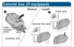
The console box can be removed and installed between the front or second row seats.
