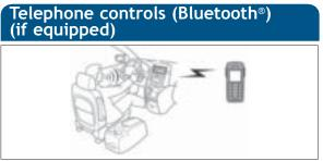
Bluetooth<sup>®</sup> technology allows dialing or receipt of calls without taking your hands from the steering wheel or using a cable to connect the telephone and the system.
