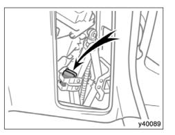
Before removing the jack, take out the adapter socket. The adapter socket is inside a bag and stored in the side of the jack, as shown in the illustration.
