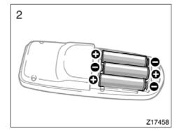
2. Remove the discharged batteries and put in the new batteries as shown. Install the cover.
