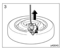
3. After the tire is lowered completely to the ground, remove the holding bracket.
