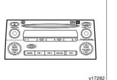
Type 2–2: AM·FM radio/compact disc player with changer (with XM $^{\odot}$  Satellite Radio\* controller)
