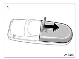
1. Remove the cover of the remote control as shown.
