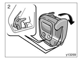
2. Make sure the front leg is locked securely, fold down the seat and engage the rear leg lock.
