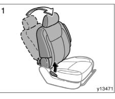
1. Pull the seatback angle adjusting lever and raise the seatback to its upright position.
