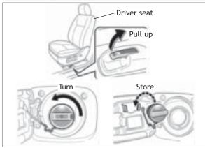
**NOTE:** Tighten until one click is heard. If the cap is not tightened enough, Check Engine " "" indicator may illuminate.
