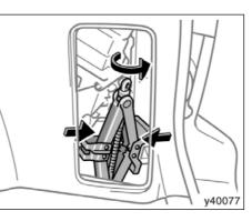
To remove the jack, turn the jack joint by hand until the jack becomes free.
