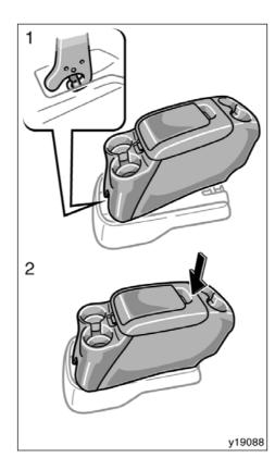
To install the console box between the front seats:
