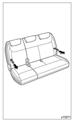
Lean forward and pull the strap forward. Then lean back to the desired angle and release the strap.
