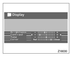
Operate the joystick up and down to select Brightness, Contrast, Tone, or Color and left and right to make adjustments.
