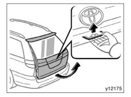
To open the back door, push up the back door opener and raise the door.
