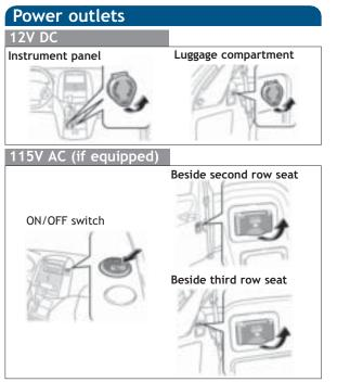
Designed for car accessories. Engine switch must be in the "ACC" or "ON" position to be used.
