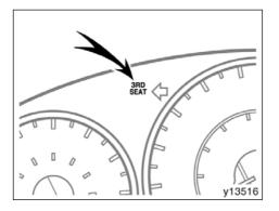
This "3RD SEAT" warning light warns the third seat operation is not yet complete when the engine switch is turned to the "ON" position.
