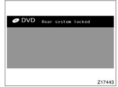
When the rear system lock is on and any button is pushed on the remote control or the operation panel, the screen shown above is displayed for approximately 6 seconds.
