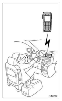
This system supports Bluetooth<sup>®</sup>, a wireless system that allows you to make or receive calls without taking your hands from the steering wheel and without using cables to connect the phone and system.
