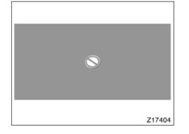
If " $\otimes$ " appears on the screen when you select a switch, it indicates that the switch cannot work.
