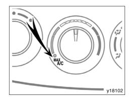
For quick cooling, turning the temperature selector knob fully towards COLD changes the air intake selector mode to RECIRCULATE. It is not possible to return to FRESH and to turn the air conditioning system off in this position.
