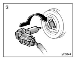
3. Plug in a new bulb into the connector and install it into the mounting hole.
