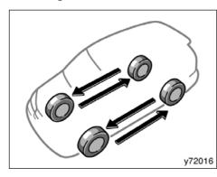
When rotating tires, check for uneven wear and damage. Abnormal wear is usually caused by incorrect tire pressure, improper wheel alignment, outof-balance wheels, or severe braking.
