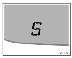
The compass indicates the direction that the vehicle is heading. In the above case, it shows that the vehicle is heading south.
