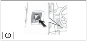
If tire pressure becomes critically low on any of the tires (excluding spare), indicator comes on. Pushing " 🔄 SET" button should not turn off the light. Correctly adjusting tire inflation will turn off the light after a few minutes. After replacing/rotating tire or wheels, the system must be initialized.
