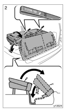
2. Pull and hold the seat lock release strap ("TO STOW/USE" printed on its surface) and lift up the seat rearward. Then push the seat down.
