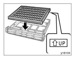
**5. Install the filter to the filter case.** Position the filter and the case so that the "<sup>↑</sup>UP" mark is pointing up.
