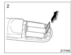
2. Remove the insulating sheet.
