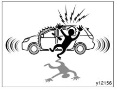
The system sounds alarm and flashes lights when forcible entry is detected. The alarm is triggered if any of the side doors, back door or hood is forcibly unlocked or opened or the battery terminal is disconnected and then reconnected when the vehicle is locked.
