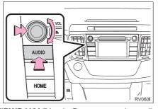
"**PWR VOL**" knob: Press to turn the audio system on and off. The system turns on in the last mode used. Turn this knob to adjust the volume.
