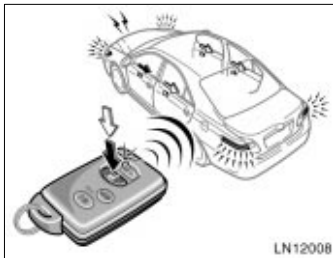
Unlocking operation (vehicles with smart key system)
