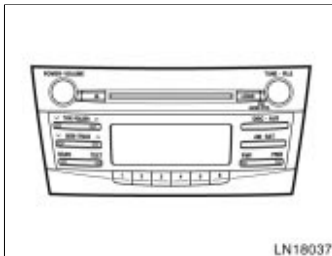
Type 2: AM-FM radio/compact disc player with changer (with XM satellite radio controller)
