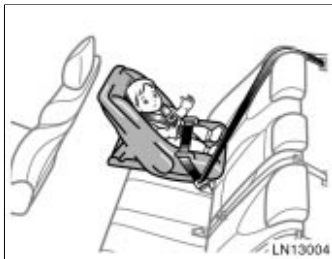
(A) INFANT SEAT INSTALLATION An infant seat must be used in rear-facing position only.
