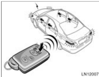
Locking operation (vehicles with smart key system)
