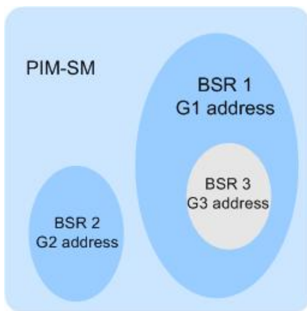
Figure 11-19 BSR Domain Divided by Multicast Address
