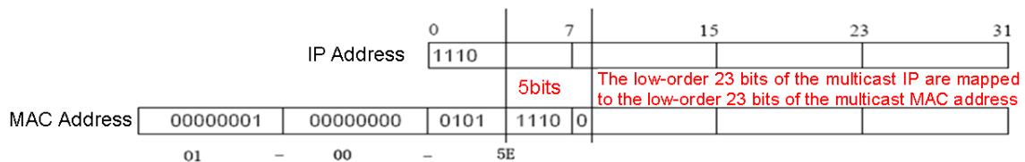
Figure 9-2 Mapping relationship between multicast IP address and multicast MAC address
