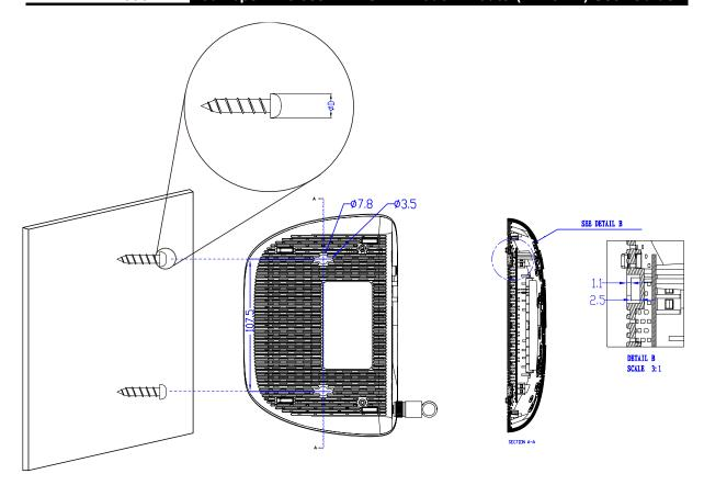
Figure 2-3 Wall-mount Install
