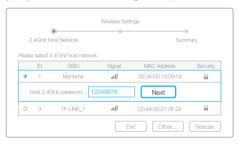
4 Either copy the host SSID or customize it for the 2.4GHz extended network, and click Next.
