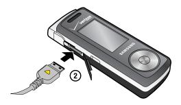
**Note:** The following illustration is the incorrect method for connecting the charger. If attempted, damage to the accessory port occurs therefore voiding the phone's warranty.
