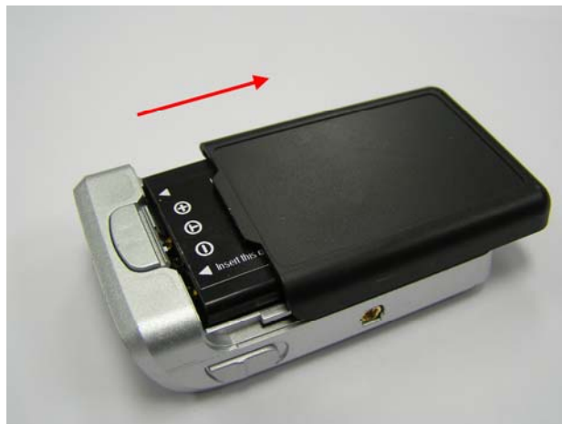
Figure 2 Open the cover of battery
