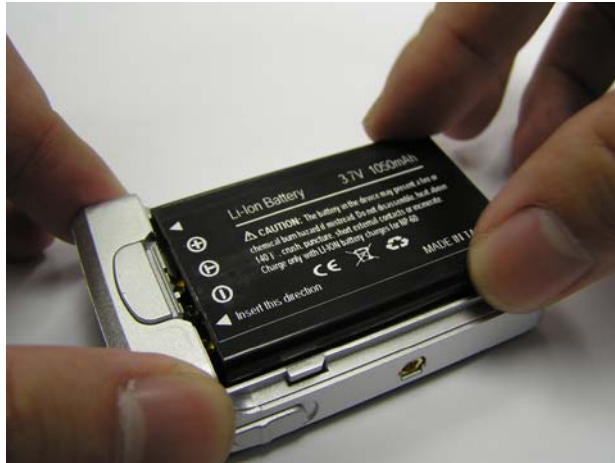
Figure 4 Fit new battery into i-Blue
