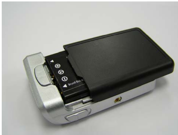
Figure 5 Slide the cover of battery to close
