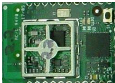
Figure 2-1. Top-Side of Trane RF Module
