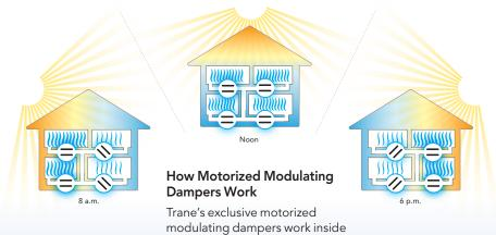
your ductwork by opening and closing in partial increments so you can fine-tune zoned areas
