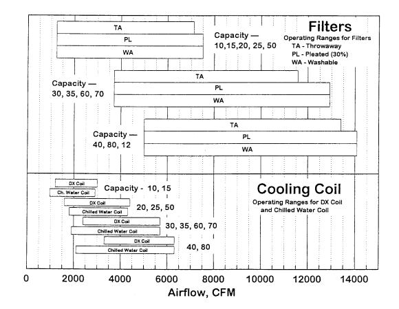
Quick Sizer Chart 4 Furnace Type (C, D) High Temperature Rise Rooftop Arrangement (G, J, K, L)
