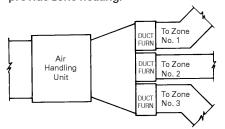
Note: When installing duct furnaces in parallel or in series, minimum clearance requirements must be considered. This clearance is required for serviceability. Duct furnaces are approved for blow-thru applications only. Right-hand burner drawers are available for parallel applications. Contact your local Trane representative for more information.
