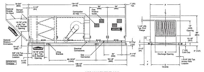
ARRANGEMENT "G" MODELS 50-80 POWER VENT (Left Hand Service Access Shown)
