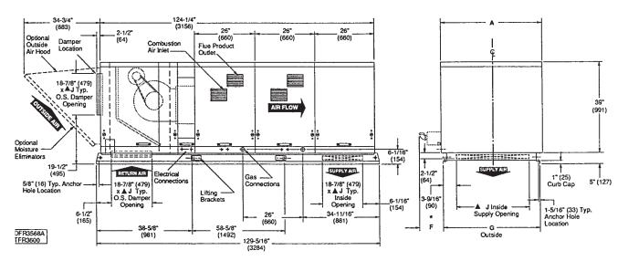
ARRANGEMENT "C" MODELS 50-80 POWER VENT (Left Hand Service Access Shown)
