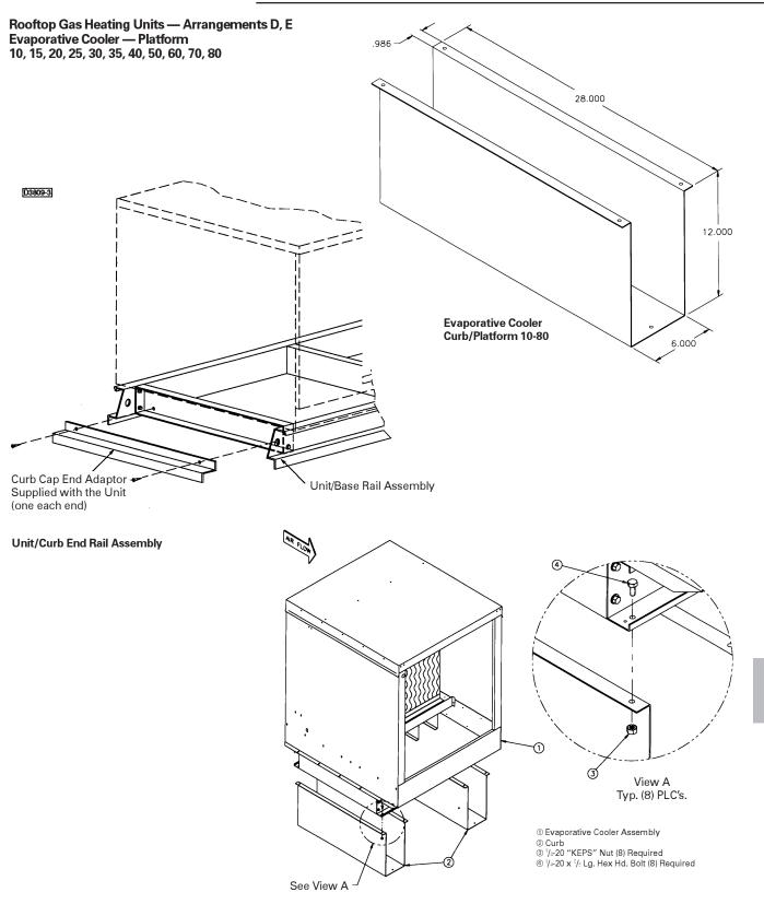
Evaporative Cooler Curb/Platform Mounting Assembly
