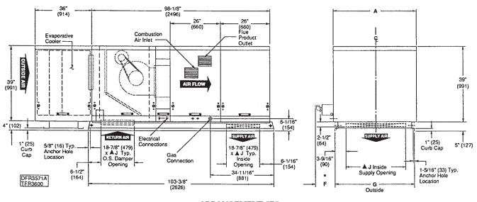
ARRANGEMENT "E" MODELS 10-40 POWER VENT (Left Hand Service Access Shown)
