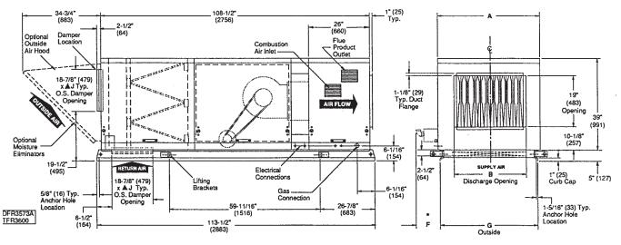
ARRANGEMENT "G" MODELS 20-40 POWER VENT (Left Hand Service Access Shown)
