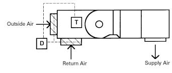
T = Temperature Sensor D = Damper Actuator
