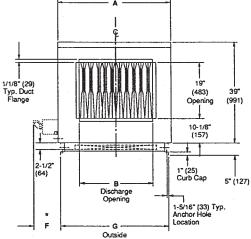
ARRANGEMENT "B" MODELS 50-80 POWER VENT (Left Hand Service Access Shown)
