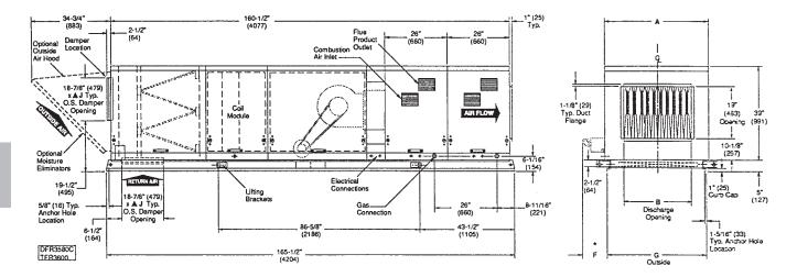
ARRANGEMENT "K" MODELS 50-80 POWER VENT (Left Hand Service Access Shown)
