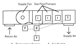
T = Temperature Sensor I = Ignition System F = Fan Switch E = Electronic Control
