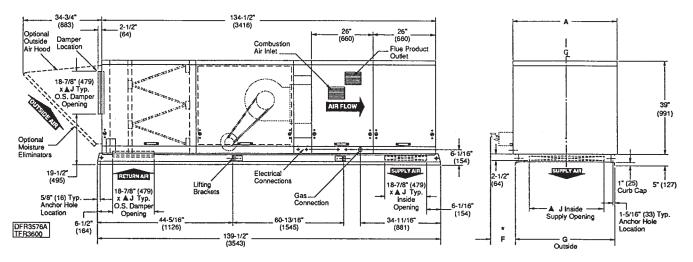
ARRANGEMENT "J" MODEL 20-40 POWER VENT (Left Hand Service Access Shown)
