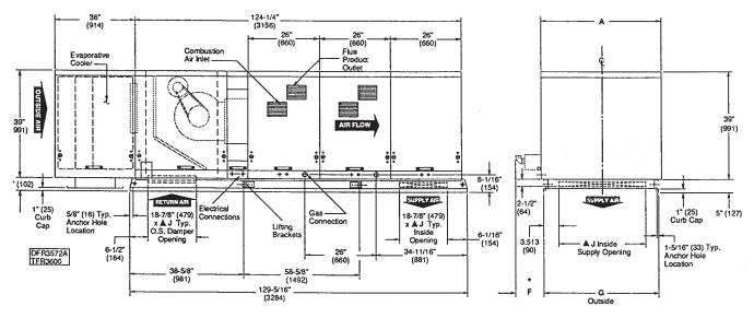
ARRANGEMENT "E" MODELS 50-80 POWER VENT (Left Hand Service Access Shown)
