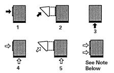
Note: Horizontal outside air over return air. Specify air inlet configuration 4 or 5 and then select miscellaneous option "D" for horizontal return.
