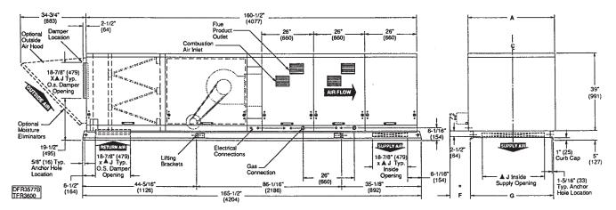
ARRANGEMENT "J" MODELS 50-80 POWER VENT (Left Hand Service Access Shown)
