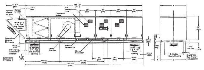
ARRANGEMENT "J" MODEL 12 POWER VENT (Left Hand Service Access Shown)
