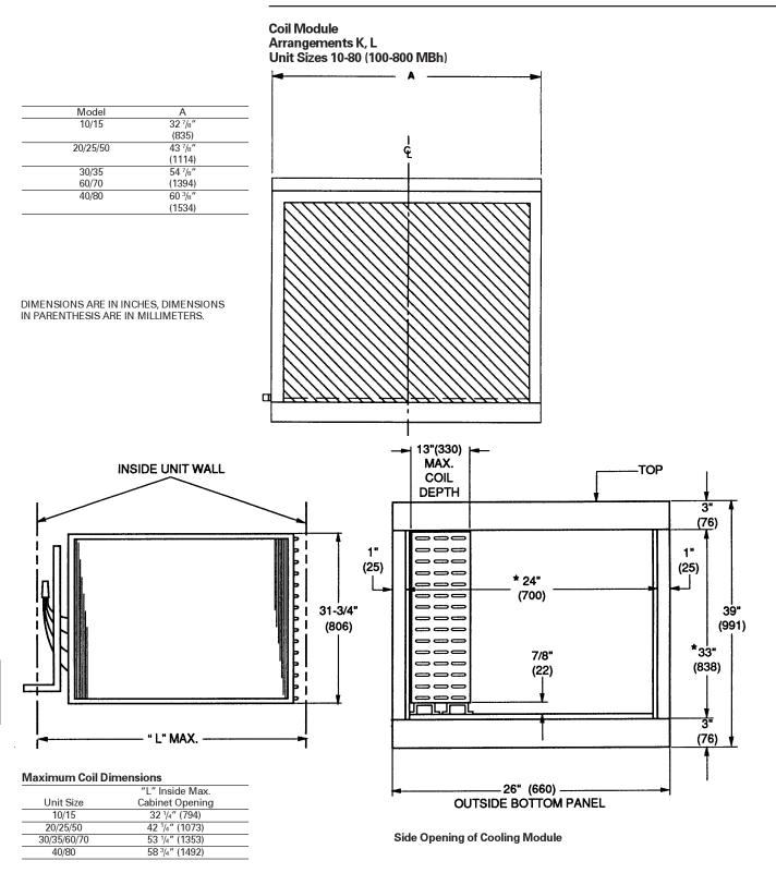
• The coil section drain pan connection is 3/4 inch NPT pipe thread. It is a female fitting that just protrudes outside of the unit base rail. It is located on the service side of the unit.
