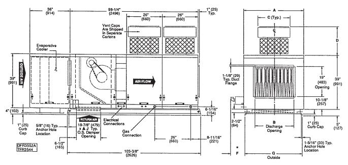
ARRANGEMENT "D" MODELS 50-80 NATURAL VENT (Left Hand Service Access Shown)
