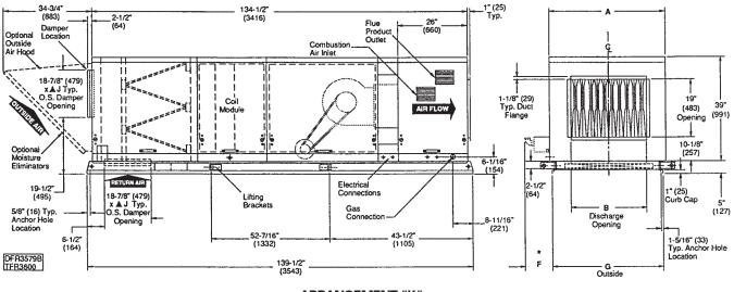
ARRANGEMENT "K" MODELS 10-40 POWER VENT (Left Hand Service Access Shown)
