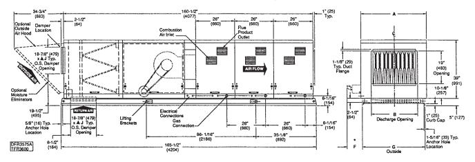
ARRANGEMENT "G" MODEL 12 POWER VENT (Left Hand Service Access Shown)
