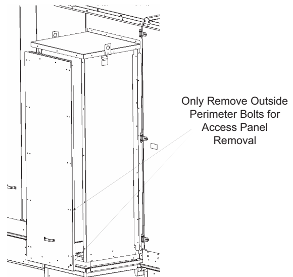
Figure 34. External piping enclosure access panel
