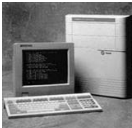
Figure 2. You can control, monitor, and service your facility using Trane's ICS and your PC
