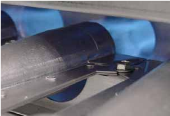
Burner flame at high fire: 3.5 in. wc manifold pressure draft inducer—high speed
