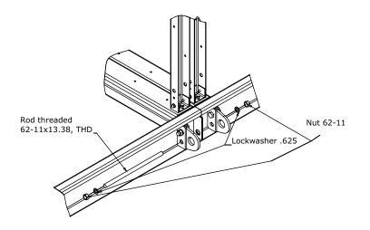
Figure 26. Insert threaded rods
