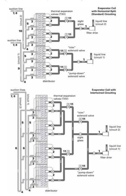
Figure 65. Dual-circuit evaporator coil with eight distributors
