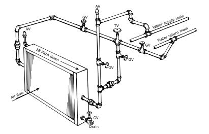
Figure 56. Typical piping for type W or WA 1-row water coil
