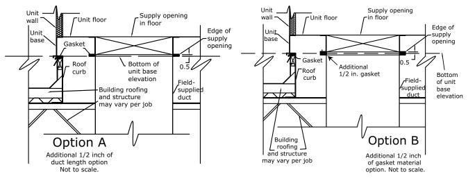
Note: Bottom of unit base elevation is 1/2 inch lower than edge of duct Note: Bottom of unit base elevation is 1/2 inch lower than edge of duct opening in bottom of unit. During unit installation on roof curb, either raise field-provided duct or add additional gasket material to compensate for the 1/2 inch offset.
