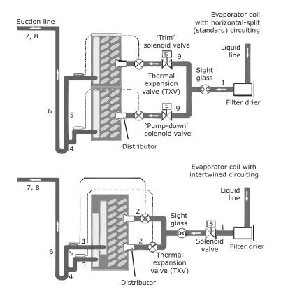
Figure 61. Single-circuit evaporator coil with two distributors
