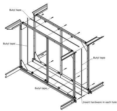
Figure 23. Butyl tape is applied to shipping splits
