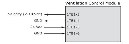
Traq dampers are low-leak dampers that modulate and measure airflow. Each Traq damper section is supplied with a factory-mounted ventilation control module (VCM) on the interior of the mixing box. The VCM has an input terminal for power and an output terminal for air velocity (see Figure 76). A direct-digital controller controls the factory-mounted and wired actuators.
