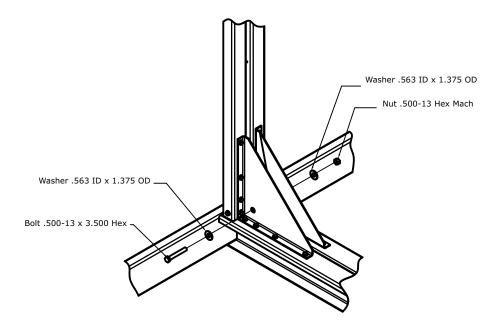
Figure 28. Join internal shipping split frame- Graphic 1
