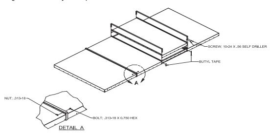
Figure 32. Trim roof joint strip
