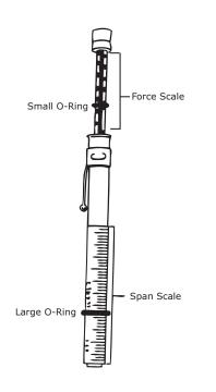
Proper belt tension is required to ensure maximum bearing and drive component life and is based on motor horsepower requirement. A label located on the bearing support on the drive side of the unit lists all drive parts, the proper belt tension, and deflection for that tension for the specific drive (Figure 72).
