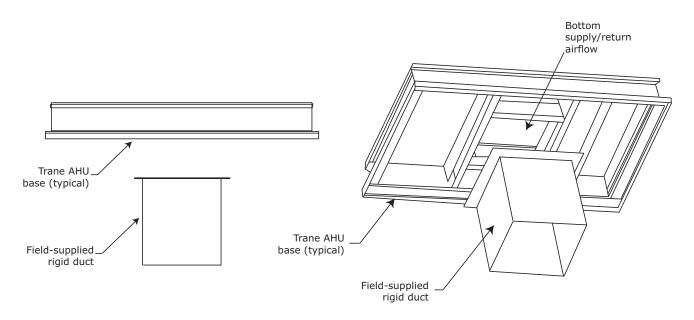
3. Bottom of unit base elevation is ½ inch lower than edge of duct opening in bottom of unit. During unit installation on roof curb, either raise field provided duct per Option A (see Figure 41) or add additional gasket material to compensate for the ½ inch offset per Option B (see Figure 42).
