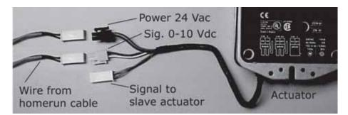
Figure 71. Typical quick connects with wiring identification
