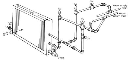
Figure 55. Typical piping for type 5A, 5W two-row, K, W 3- to 12-row, WD, D, and DD water coils
