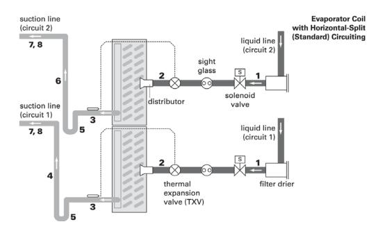
Figure 63. Dual-circuit evaporator coil with two distributors
