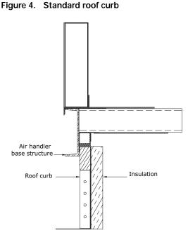
The TCP unit exterior base channel is constructed to overhang the roof curb. Unit support is provide by a square tube channel locate inside of exterior base channel. See Figure 4. The standard curb should be designed to properly support the unit's weight without bow and sized to fit within the perimeter base channel.
