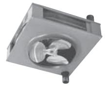
Vertical units are available in fifteen sizes for steam or hot water heating. Steam capacities range from 140 to 2,580 E.D.R. (26.0 to 705 MBH) (2 PSI w/60° E.A.T.). Hot water capacities range from 18.9 to 519.4 MBH (200° E.W.T./20° drop w/60° E.A.T.).
