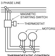
THERMOSTATIC CONTROL **OF SEVERAL THREE PHASE UNITS** Figure 14.
