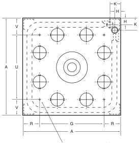
(4) MOUNTING HOLES 3/8 - 16 FOR 102P-384P THREAD TAPS 1/2 - 13 FOR 500P-720P
