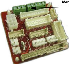
**Note:** Customer Low-Voltage Interface for Fan Speeds, Variable Fan Speed, and 24 Vac Supply
