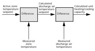
If the discharge air temperature falls below the discharge air temperature low limit setpoint, (configurable using the Tracer TU service tool), and the cooling capacity is at a minimum, the available heating capacity is used to raise the discharge air temperature to the low limit.
