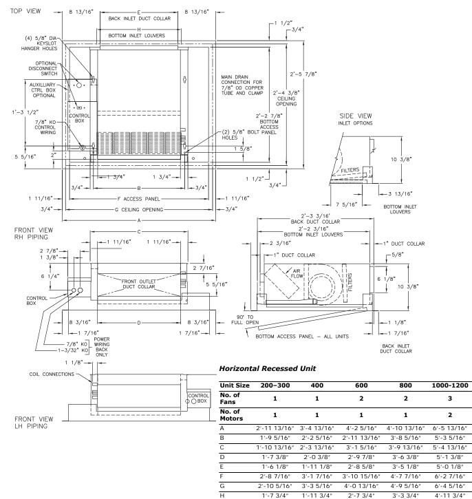
1. Coil connections are always opposite the drain pan side.
