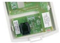
Figure 16. Split-mounted zone sensor, unit-mounted fan mode and wall-mounted setpoint dial: Digit 30 = F, G, or J and Digit 31 = Y
