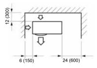
When top of unit is blocked and the air outlet is opposite the wall
