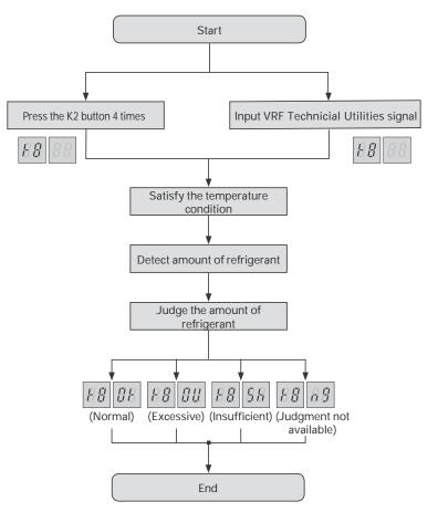
After the refrigerant detection operation is complete, take the following actions:
