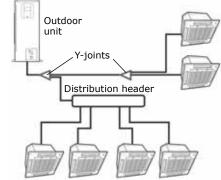
Example with Y-joints and distribution header
