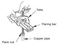
5. Remove the pipe. The end of the pipe that you flared should look like the end of a trumpet. See examples of correctly and incorrectly flared pipes.
