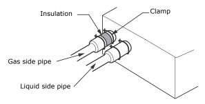
4. Cut off excess insulation.
