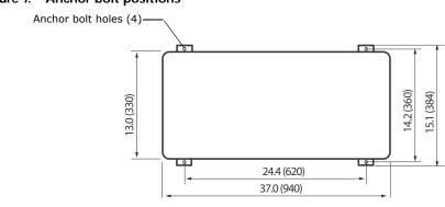
Figure 7. Anchor bolt positions
