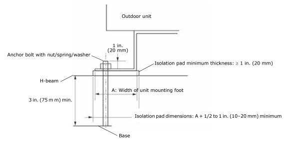
After installing a vibration-isolation frame, loosen the bolts so that the isolators are capable of absorbing vibrations (Figure 6).
