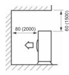
When from and back of unit are blocked by walls
