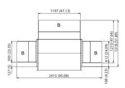
A: Optional condenser air discharge duct B: Optional wind/snow protection duct
