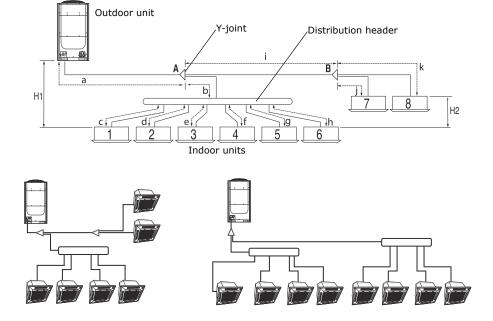
Figure 15. Single installation with Y-joint and distribution header: Heat pump
