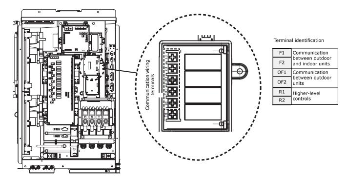
To provide strain relief, secure the communications cable with a clamp in the location shown in Figure 27.
