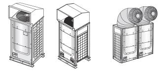
Examples of condenser air discharge ducts
