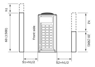
Front wall height recommendation: 60 in. (1500 mm) maximum. Back wall height recommendation: 20 in. (500 mm) maximum. Side wall height is unlimited.
