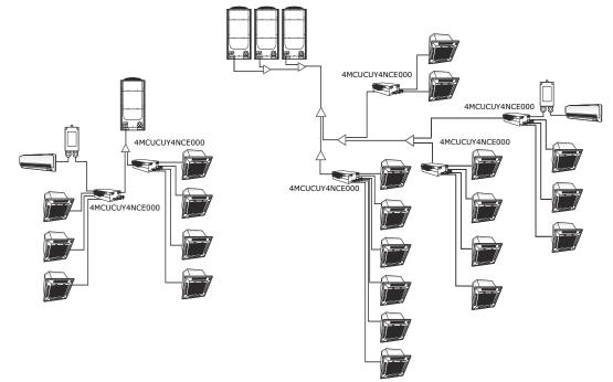
Figure 20. Installation with MCU: Heat recovery
