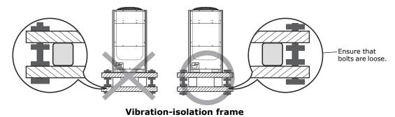
After installing a vibration-isolation frame, loosen the bolts so that the isolators are capable of absorbing vibrations (refer to the figure below).
