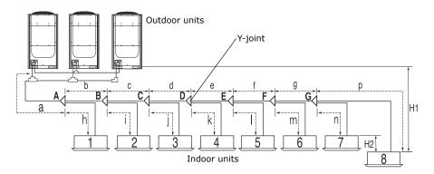
Figure 17. Module installation with distribution header: Heat pump
