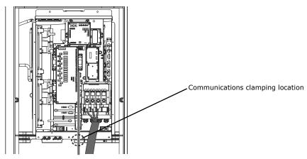
Figure 27. Communications cable clamping location
