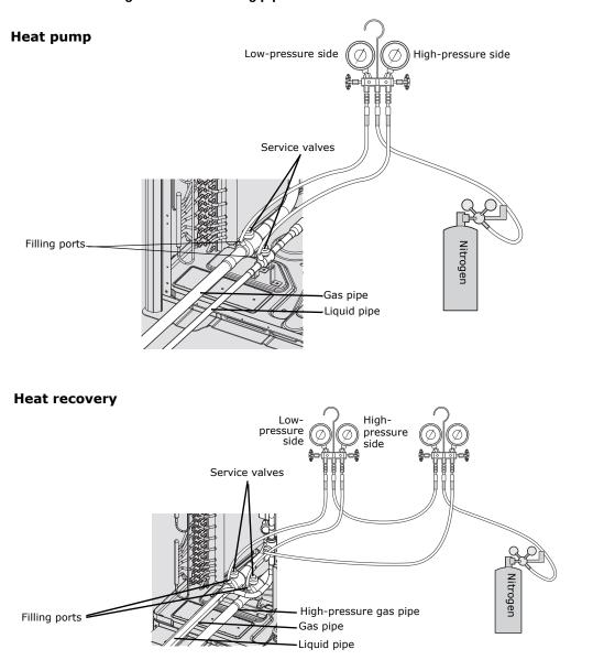
Use the following procedure for leak testing pipe connections. Refer to Figure 28.
