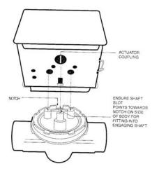
4. Install body valve into pipe.
