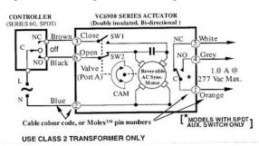
The typical floating controller is an SPDT controller with a center-off position. On a change in temperature from the set point, the controller will close the normally open (NO) or normally closed (NC) contacts, driving the valve to an intermediate position until a further change at the controller.
