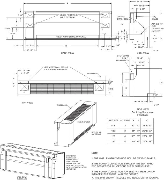
4. THE UNIT SHOWN INCLUDES THE INSULATED HORIZONTAL BAFFLE OPTION.
