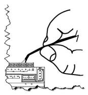
To connect wires to the UC400 controller or the expansion modules:
