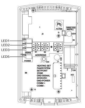
The sensor for model WZS have four LEDs: LED1, LED2, LED3, and LED5. The sensor for model WDS has test symbols and error codes that appear on the display. All three sensor models have a Test button. Figure 66 shows their locations.
