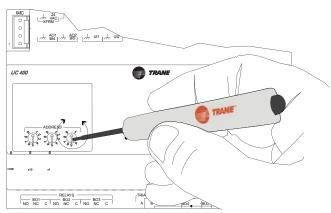
Use a 1/8 inch (3.2 mm) flathead screwdriver to set rotary address dials. Dials rotate in either direction.
