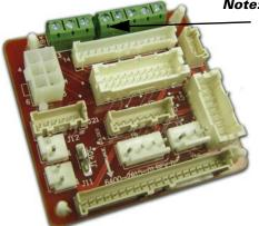
Note: Customer Low-Voltage Interface for Fan Speeds, Variable Fan Speed, and 24 Vac Supply
