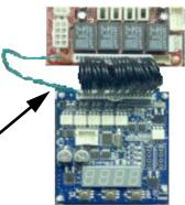
Green wire attached to white plug on blue ECM engine board, and to quick-connect terminal on the adapter board.
