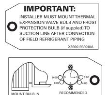
Note: Depending on the controls package ordered with the unit, not all installations will require mounting the frost stat bulb.
