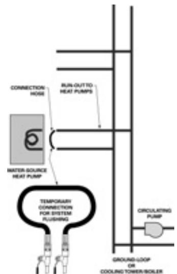
Figure 6: System flushing
