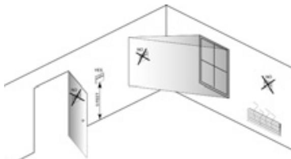
Figure 7: Thermostat/sensor location
