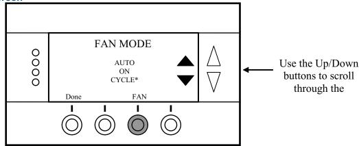
Normally the FAN mode is in the Auto mode (the system fan is automatically controlled by HVAC system). If you want the FAN on manually, select the ON mode. The fan will run continuously until it is turned to off by selecting AUTO mode.
