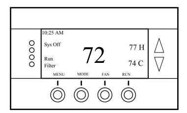
The main Thermostat Control Screen is the default display screen and is the screen that is normally displayed on the Thermostat.
