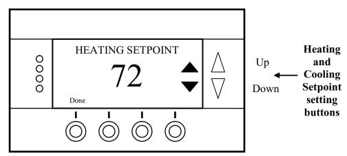
The UP and DOWN buttons adjust the setpoint temperature. Pressing the UP button will increment the setpoint value by one degree and conversely, pressing the Down button will decrement the setpoint one degree. Pressing and holding a button down will cause the setpoint to continuously change until the button is released.
