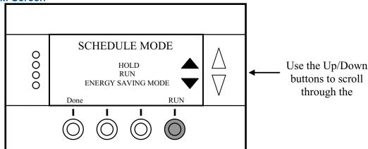
Run Mode. In the run mode, the thermostat schedule is running and setpoints will change according the times and temperatures in the schedule. The schedule can be local (if enabled in the Installer Settings) or remote via the Z-Wave network.
