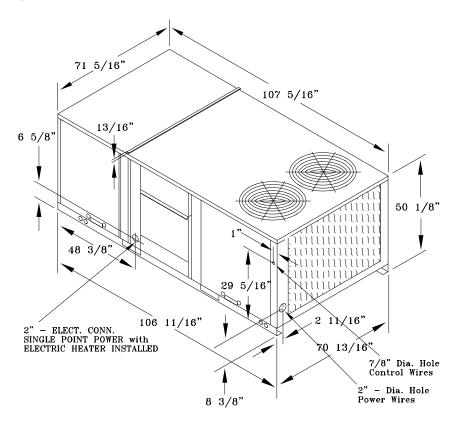
Figure 2. Unit Dimensional Data 12 1/2 Ton, 15 Ton
