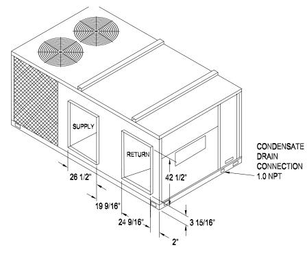
Figure 6. Horizontal Duct Dimensional Data 12 1/2 Ton, 15 Ton
