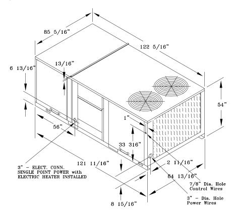
Figure 4. Unit Dimensional Data 20 Ton
