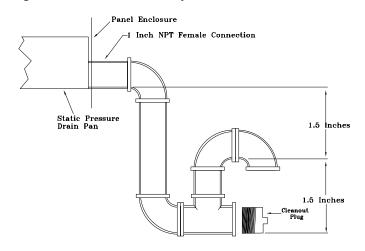
Figure 9. Condensate Trap Installation
