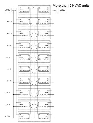
Figure 13. Typical field wiring diagrams for optional controls (ReliaTel™ only)
