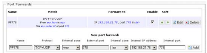
Figure 61: Adding a port forwarding rule.
