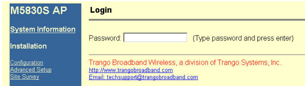
Figure 4-3: Browser Interface Login Page Type the password (default trango ) and continue. This will bring up the radio's System Information page.
