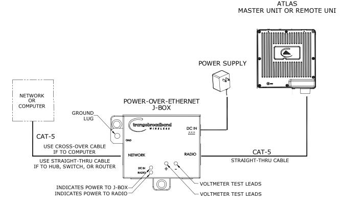
Both green LEDs on the J-box should be lit, indicating power is present at the Power-over-Ethernet box as well as at the radio.
