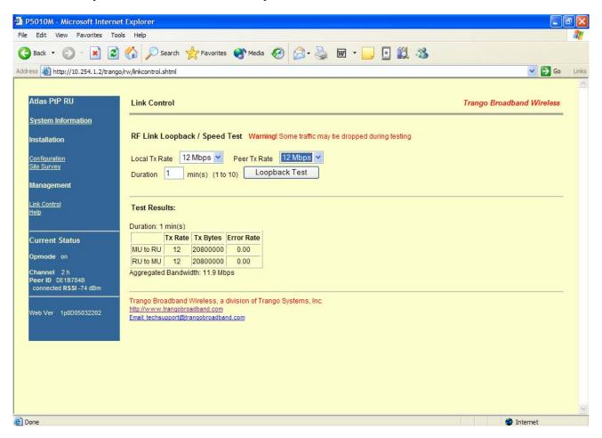
In this example, the error rate was 2 packets from MU to RU and 0 packets from RU to MU. Measured aggregate bandwidth is 10.93 Mbps.
