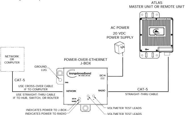
Both green LEDs on the J-box should be lit, indicating power is present at the Power-over-Ethernet box as well as at the radio.
