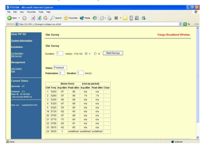
In this example the site survey function was performed for 1 minute on the vertical polarity. The lower band (5250 – 5340 Mhz) is reported to be relatively clean with a noise floor in the range of –97 to –98 dBm. The noise floor in the upper band (5735 – 5835 MHz) is higher and ranges from –58 dBm (at 5735 Mhz) to –90 dBm (at frequency 5775 MHz. In this example, channel 19 is the noisiest and should be avoided.
